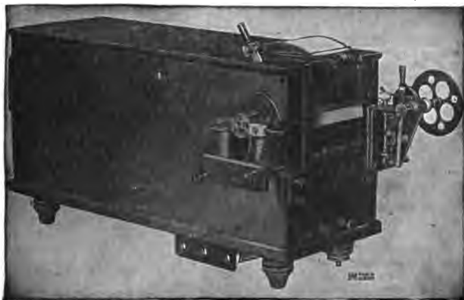
FIG. 2,600. —General Electric moving coil oscillograph. The moving elements consist of single loops of flat wire carrying a small mirror and held in tension by small spiral springs. The current passing down one side and up the other, forces one side forward and the other backward, thus causing the mirror to vibrate on a vertical axis. The vibrator elements fit into chambers between the poles of electro-magnets, and are adjustable, so as to move the beam from the mirror, both vertically and horizontally. A sensitized photographic film is wrapped around a drum and held by spring clamps. The drum, with film, is placed in a case and a cap then placed over the end, making the case light, when the index is either up or down. The loading is done in a dark room. A driving dog is screwed into the drum shaft, and which, when the drum and case are in place, revolves the film past a slot. When an exposure is to be made, the index is moved from the closed position, thus opening the slot in the case and exposing the film to the beam of light from the vibrating mirrors when the electrically operated shutter is open. The slot is then closed by moving the index to "Exposed." A slide with ground glass can be inserted in place of the film case or roll holder to arrange the optical system when making adjustments. The shutter operating mechanism is arranged so as to hold the shutter open during exactly one revolution of the film drum. There are two devices connected to the shutter operating mechanism; one opens the shutter at the instant the end of the film passes the slot; the other opens immediately, at any part of the film, and both give exposure during one revolution. The first is useful when making investigations in which the events are either recurring, or their beginnings known or under control, and the second when the time of the event is not under control, such as the blowing of fuses or opening of circuit breakers.
