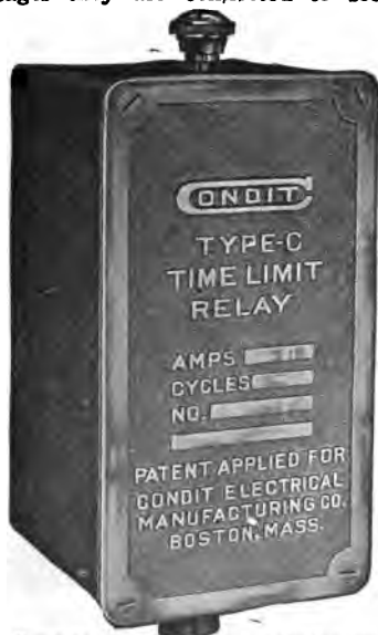
FIG. 2,342. —Condit time limit relay, designed primarily for use in connection with feeder circuits, where close selection or discrimination of circuit breakers is not required. It may be used satisfactorily on lighting and power circuits and also where there are sudden, momentary fluctuations of current. This relay is used in connection with series transformers. The contact arrangements are provided so that the relays may be used as circuit closing or circuit opening relays. The delayed action is produced by an air vacuum dash pot with a graphite piston. The piston of the dash pot is connected to an arm arranged to be moved by the armature. When the current reaches a point where it overcomes the weight of the armature and lifts the same, the magnetic force tending to lift the armature is opposed by the pull of the vacuum created in the interior of the shell into which fits the graphite piston. As the magnetic pull continues the vacuum is overcome due to the leakage of air past the piston, and the armature gradually moves until it reaches a point where it causes the circuit breaker to trip, either by closing the contacts in the circuit closing type, or by opening the contacts in the circuit opening type. If, at any portion of its travel, the current drop to normal, the armature immediately resets. The time adjustment consists of an arrangement whereby the distance through which the armature moves before tripping the breaker, may be changed, thus altering the time of tripping. The current adjustment is made by changing the effective turns of the actuating coil, the travel of the armature and the force exerted by it being the same for all current adjustment. The winding is designed to carry 5 amperes continuously with a temperature rise not exceeding 68° Fahr. standard calibration is provided so that the relay will start to operate at 5, 6, 8 and 12 amperes.
