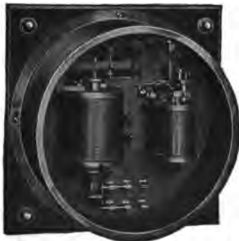
FIG. 2,424. —General Electric direct current (form S) voltage regulator. It consists of a main control magnet, relay, condenser and reversing switch, as shown in the diagram fig. 2,423. This regulator cannot be used for compensation of line drop as the current coil is omitted; it is not a switchboard instrument, but is designed for inexpensive installations such as for regulating the voltage of motor generator sets when the current is taken from a trolley line or some other fluctuating source. The regulating outfit comprises, besides the regulator, one or more condenser sections according to field discharge, set of iron brackets when regulator cannot be mounted on front of switchboard, one compensating shunt, when it is desired to compensate for line drop. Field rheostats having sufficient resistance to reduce the voltage the proper amount must be used with voltage regulator installations. To prevent undue decay at the relay contacts, allow one section for each 15 kw. capacity of dynamo with laminated poles, and one for each 22 kw. capacity with solid steel poles.
