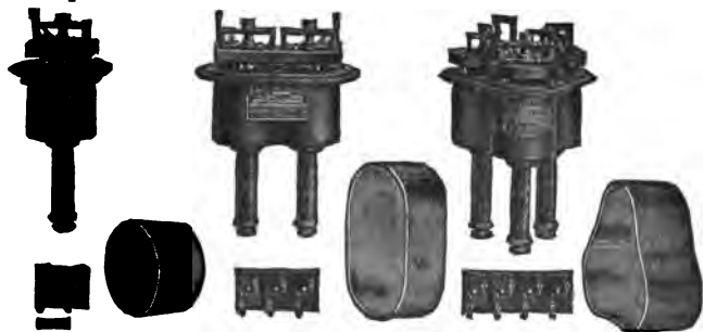
Figs. 2,283 to 2,291. —General Electric instantaneous overload circuit opening relays, covers removed. Circuit opening relays are used chiefly in those cases where direct current for the tripping circuit is not available. Alternating current trip coils have relatively high impedance and impose a heavy volt ampere load on the current transformers. To reduce this load during normal operation the circuit opening relay is frequently used and is usually necessary where instruments and meters are to be operated on the same current transformers as the trip coils if the greatest accuracy be required. The relay contacts in the normal, closed position, short circuits the trip coil. When the relay operates on overload or other abnormal condition the contacts are opened with a quick break, sending the current through the trip coil circuit momentarily and tripping the switch. With circuit opening relays, the trip coils of the oil switch must be set to trip somewhat lower than the setting of the relay. In construction the relay consists of a solenoid with iron frame forming the support for the relay; a central plunger or armature of special construction which is picked up or released by the magnetic action of the solenoid; a plunger rod which actuates the relay contacts, which are mounted on an insulated base usually above the solenoid; a tube or plate for the calibration marking and adjustment; covers of glass or metal to keep out dust; terminal boards with points corresponding to tagged leads from relay coils and external wiring diagrams. The relay contacts are of two kinds, circuit opening, as shown above, and circuit closing, as shown in figs. 2,292 to 2,300.
