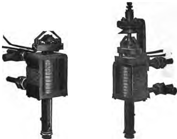
Figs. 2,311 and 2,312. —General Electric alternating current low pressure series overload relays. Fig. 2,311, instantaneous time limit relay; fig. 2,312, inverse time limit relay. These relays have carbon contacts and will make or break a direct current circuit of 10 amperes at 125 volts without auxiliary circuit opening switch. They are used where several circuits are controlled by one automatic oil break switch or one shunt trip, overload and shunt trip or low voltage release carbon break circuit breaker. These relays may be used for signal purposes; they are back connected, the connections can be seen in the illustrations.
