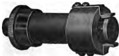
FIG. 2,273 —General Electric circuit opening auxiliary switch . This switch opens an auxiliary circuit when the circuit breaker opens, and is intended to be used in connection with a shunt trip attachment to insure the immediate disconnection of the shunt coil from the circuit. It may also be employed to serve other purposes, such as tripping another circuit breaker having a low voltage attachment, and permitting another circuit breaker to remain closed only when the circuit breaker equipped with the auxiliary switch is open.
