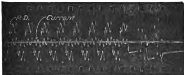
FIG. 2,625. —Portion of oscillograph record taken with a cinematograph film camera showing the effect of switching off a high pressure feeder and illustrating the violent fluctuations produced by sparking at the switch contacts.
