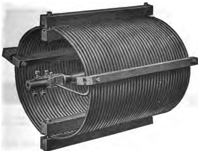
FIG. 2,406.—Westinghouse line suspension choke coil. It is so designed that it can be inserted directly in the transmission line wire or in the station wiring and held in position therein by the tension of the line or station wires. Because of the fact that no insulators are required, solely to support this choke coil, and that it can be installed in either a vertical or a horizontal position it can often be utilized effectively in power and substation layouts. Terminals, each having a \frac{1}{2} inch round hole, to accommodate the conductors are provided at each end of the coil. Three square headed binding screws are supplied which clamp the conductors in position. The coil is provided with a strain insulator, so arranged within the coil at its axis, that it assumes any mechanical tension transmitted from the conductors. No mechanical tension reaches the turns of the choke coil proper. In construction, the choke coil is made in but one size having a current carrying capacity of 200 amperes and is suitable for a voltage of 2,000 to 22,000. For higher voltages than 22,000, several choke coils are connected in series. One coil is used for each 22,000 volts or fraction thereof, of the pressure between the wires of the circuit. Application: This type of choke coil may be used for alternating current service for the entire range from 22,000 to 110,000 volts. It may be used on transformers, but is not recommended for the protection of generators.
