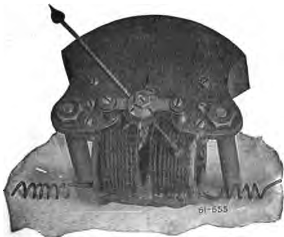
FIG. 2,514.—Wagner dynamometer movement. In this type of instrument the deflection is proportional to the square of the current, producing a constantly decreasing sensitiveness as the pressure applied is decreased. The dynamometer movement is, for any indication, more accurate than the magnetic vane, but cannot readily be employed for the indication of current, as required in ammeters.
