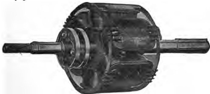
FIG. 2.481. —Field of a synchronous condenser. Note the amortisseur winding, erroneously called squirrel cage winding, consisting of two end rings which serve to short circuit spokes passing through the pole tips as shown. The amortisseur winding assists in starting and serves also as a damping device to minimize hunting.
