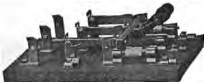
FIG. 2,206.—Westinghouse fused starting switch for squirrel cage motors. It is arranged for National Electric Code fuses on one end only and has springs on the other end to open the switch automatically if left closed at this end. The corresponding terminals at both ends of the switch are connected in grooves in the back of the slate base so that the wiring need be connected to one set of these terminals only, thus decreasing the number of connections necessary, as shown in fig. 2,207. In starting an induction motor, the switch is thrown to the end that is not fused and held there until the motor is up to running speed; then it is quickly thrown to the fused position, thus protecting the circuit under running conditions.
