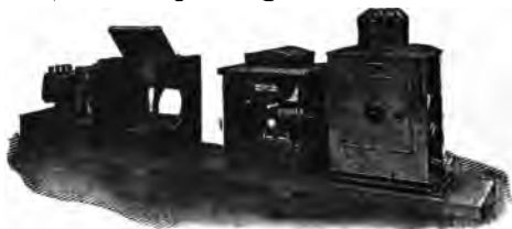
FIG. 2,613.—Duddell moving coil oscillograph with projection and tracing desk outfit. The outfit is designed for teaching and lecture purposes. In operation, after the beam of light from the arc lamp has been reflected from the oscillograph mirrors, it falls on a vibrating mirror which gives it a deflection proportional to time in a direction at right angles to the deflection it already has and which is proportional to the current passing through the oscillograph. It is therefore only necessary to place a screen in the path of the reflected beam of light to obtain a trace of the wave form. Since the vibrating mirror is vibrated by means of a cam on the shaft of a synchronous motor, which motor is driven from, or synchronously with, the source of supply whose wave form is being investigated, the wave form is repeated time after time in the same place on the screen, and owing to the "persistence" of vision, the whole wave appears stationary on the screen. The synchronous motor with its vibrating mirror, mentioned above, is located underneath the "tracing desk." When used in this position a wave a few centimeters in amplitude is seen through a sheet of tracing paper which is bent round a curved sheet of glass. A permanent record of the wave form can thus easily be traced on the paper. A dark box which is designed to hold a sheet of sensitized paper in place of the tracing paper, can be fitted in place of the tracing desk. Thus an actual photographic record of the wave form is obtained. If the synchronous motor be transferred from its position underneath the tracing desk to the space reserved for it close to the oscillograph, the beam of light is then received on a large mirror which is placed at an angle of about 45 degrees to the horizontal and so projects the wave form onto a large vertical screen which should be fixed about two and a half meters distant. Under these conditions a wave form of amplitude 50 cm. each side the zero line may be obtained which is therefore visible to a large audience.
