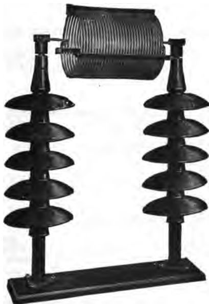
FIG. 2,412. —Westinghouse air cooled choke coil, for voltages of from 2,200 to 110,000. In construction, the coils are made of aluminum rod wound into a helix of about 15 inches in diameter and having 20 turns. The helix is supported on two insulators. For mechanical reasons it is necessary to have the aluminum rod of sufficient size to secure rigidity, consequently every coil has a capacity of 200 amperes and may be used on any circuit up to that capacity. The coils are insulated according to the standard practice for disconnecting switches, the insulators being mounted on wooden pins supported by a wooden base. This apparatus can be mounted in any position. The wiring of a station or sub-station is facilitated because the protection may be placed so as to simply form part of the wiring. The coils are symmetrical so that it is immaterial which end is connected to the line or to the apparatus.
