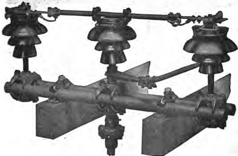
FIG. 2,214. —Baum 35,000 volt, 200 ampere, double break pole type switch. While designed for disconnecting purposes only, it can break considerable amperage. The levers and couplings are fastened with tape pins. The control shaft coupling is adjustable to any angle, and the switch can be locked in the open or closed position. A removable wooden handle is supplied and the switch can be handled in any weather. The arms can be extended to hold fuse fittings, or dead end insulators in the event of a heavy strain, but it is preferable to have fuses on another structure as a precaution against coming in contact with the energized portion of the switch, and it is also preferable to take the strain of the line on a pole a few feet from the switch, rather than on the switch structure, particularly in the larger sizes. An insulating wood section in the control shaft separates the control handle from the remainder of the switch. Discharging horns can be fitted to this type of switch and when so equipped they have been found capable of breaking considerable loads.
