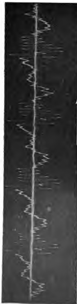
FIG. 2,633.—Current wave in telephone line corresponding to sustained vowel sound "i," as in machine; voice pitched at A 110.
