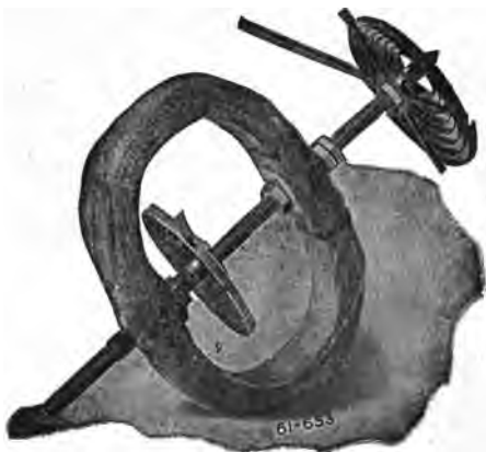
FIG. 2,515. — Armature of Wagner dynamometer movement. Greater accuracy is claimed for this movement than the magnetic vane, but it cannot readily be employed for the indication of current flow, as required in ammeters. The magnetic vane movement is used on the A. C. ammeter, and can be used also in the A. C. voltmeters; it makes use of its controlling spring only for the purpose of resisting the pull on the vane and the returning of the pointer to zero. The dynamometer movement is recommended for voltmeters.
