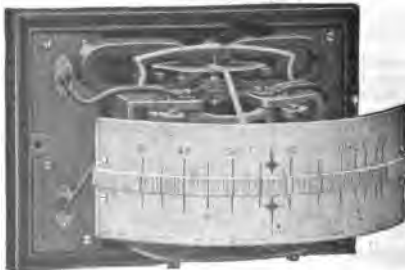
FIG. 2,569.—General Electric horizontal edgewise, induction type frequency indicator. It is provided with an external inductance and resistance placed in a ventilated cage for mounting on the back of the switchboard. Means are provided for adjusting the instrument for the characteristics of the circuit on which it is installed. Standard instruments are wound for 100 to 125 volt circuits only, but can be wound for circuits up to and including, 650 volts. Instruments for use on circuits in excess of 650 volts are always provided with pressure transformers. The normal operating point is marked at approximately the center of the scale, thus giving the advantage of very open divisions. The standard frequencies are 25, 40, 60, 125 and 133.
