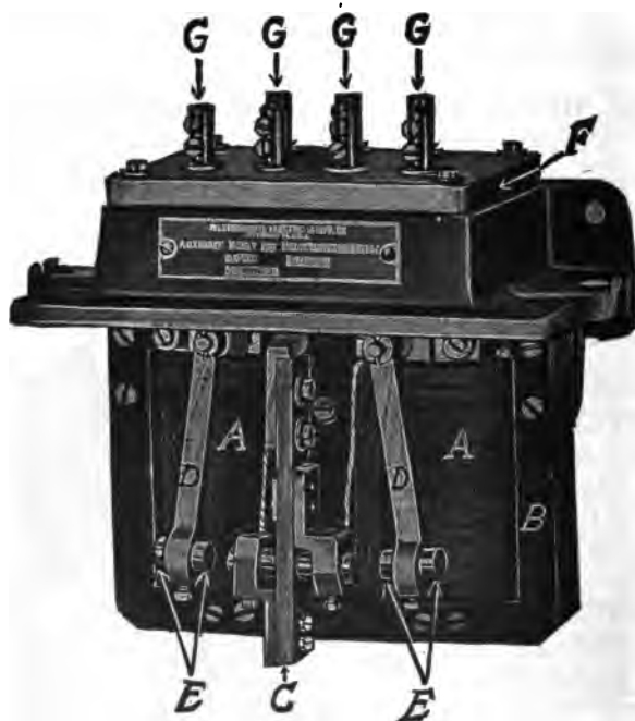
FIG. 2,427.—Westinghouse voltage regulating secondary relay; view showing relay removed from oil tank. The secondary relay is practically a motor starting switch of the double pole double throw type, electrically operated through the contacts of the primary relay. It is provided with contact points of one-half inch rod. The relay is suitably connected for starting, stopping and reversing the motor and for properly operating the motor brake. The parts are: A, solenoid; B, laminated field; C, movable contact arm; D, stationary contact arms; E, removable brass contact points; F, terminal block; G, terminals.
