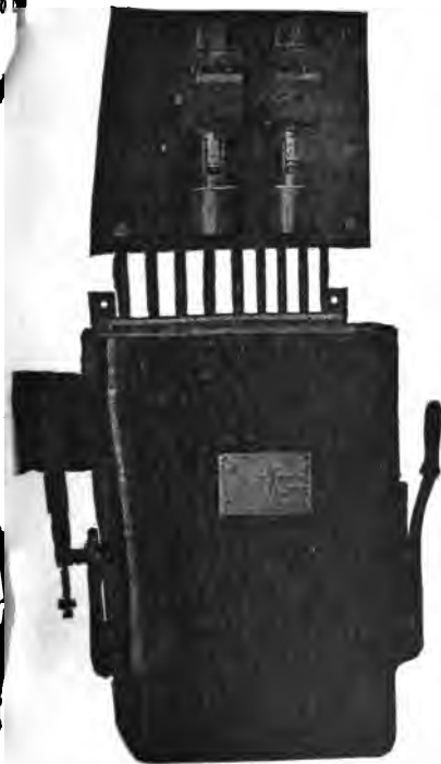
FIG. 2,469. —General Electric starting compensator with low voltage release and overload relays. On the switch shaft there are mounted two levers, held together with a strong spring which operates in either direction and prevents the switch being left on the starting position. On the running side it is held by the external low voltage release lever until released either by hand or by the action of a low voltage relay. The low voltage release consists of a cast iron frame open at the bottom and totally enclosing the coil. A laminated plunger is used to hold the tripping lever, the latter engaging with the lever mounted on the switch shaft. The compensator cannot be thrown into the running position without first going to the starting position and it cannot be left on the starting position.
