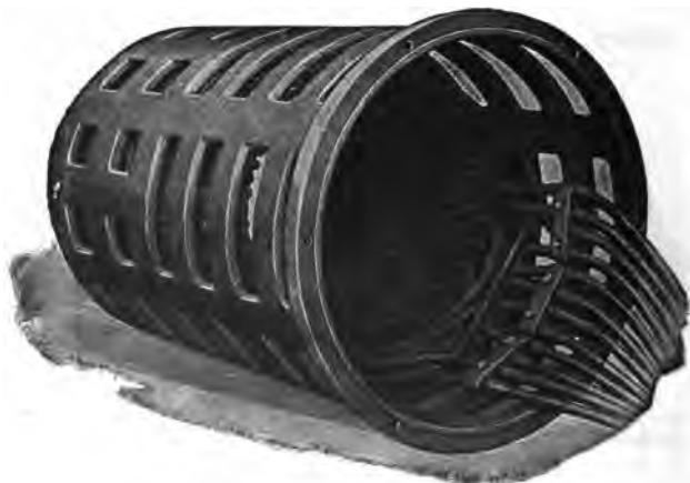
FIG. 2,419. —Top end of stationary element or secondary of Westinghouse polyphase induction regulator; view showing leads. The secondary is built up in a short skeleton frame with brackets for the rotor bearings bolted to the frame and the top cover bolted to the top brackets. In assembling the secondary, the punchings are stacked loosely in the skeleton frame and an expanding building mandrel placed inside the punchings and expanded, thereby truing up the latter before they are finally compressed and the end plates keyed in position. Then, prior to removing the mandrel a finishing cut is taken on the surface of the frame to which the bearing brackets are attached, and as the top cover and brackets are also accurately machined the alignment of the primary with the secondary is almost perfect, thus reducing to a minimum the tendency to develop vibration and noise.
