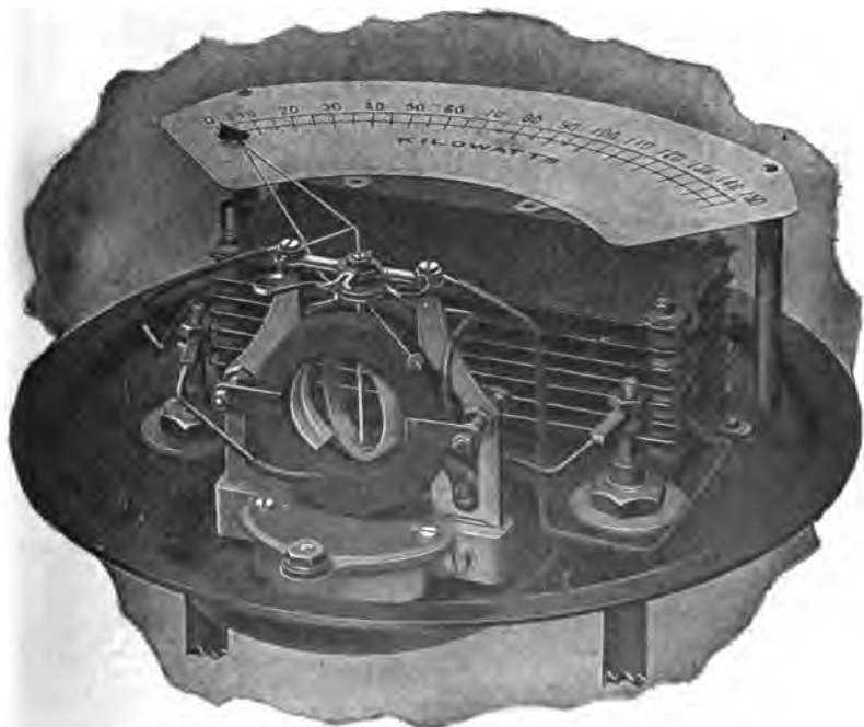
FIG. 2,527 —Interior Weston single phase wattmeter. The general appearance of the dynamometer movement and the relative positions of the various parts are clearly shown. The parts are assembled on one base, the whole movement being removable by unfastening two bolts. The fixed winding is made up of two coils, which together produce the field of the wattmeter. The movable coil is wound to gauge with silk covered wire and treated with cement. While winding, the coil is spread at diametrical points to allow the insertion of the staff, which is centered by means of two curved plates cemented to the inside surface of the coil and forming a part thereof. The coil is held in a definite position by two tiny pins which pass through the staff and engage with ears on the curved plates.
