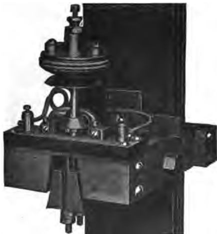
FIG. 2,340. —General Electric direct current, reverse current relay, used to protect dynamos, storage batteries, or main station busses from damage on reversal of current due to short circuits or from the grounding of machine or connections. It is mounted on vertical bus bars as in the case of cables, on the side wall, or other flat surface, and the cables threaded through the frame. When used to trip a circuit breaker, the breaker is provided with a shunt trip connected across the circuit, the tripping circuit being closed through the relay contacts on the occurrence of sufficient reverse current to lift the relay armature. The relay is either instantaneous or time limit as desired. In the time limit relay, the time interval is obtained by the leather bellows shown in the illustration. The time setting can be varied within certain limits by means of a valve on the bellows outlet. The operation of the relay depends on the relative value and direction of magnetic flux set up by a pressure coil, shown in the illustration, and the current in the vertical bars. Under normal conditions these fluxes are in the same direction and circulate around a closed magnetic circuit. When the current in the bars reverse, the two fluxes oppose each other and force flux through the normally open leg of the magnetic circuit. When the reversal of current is of predetermined value, the relay armature is lifted and the purpose of the relay accomplished.
