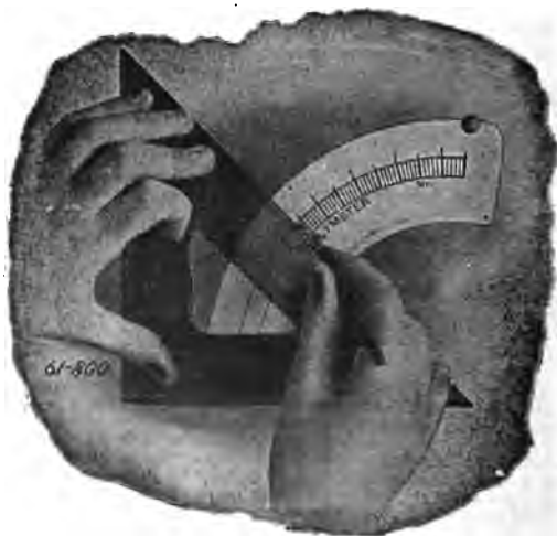
FIG. 2,495. —A calibrated scale. This means that printed scales are not employed, but each instrument has its scale divisions plotted by actual comparison with standards, after which the division lines are inked in by a draughtsman. There are makes of direct current instruments employing printed scales in which the scale deflections are fairly accurate, even though the scales are printed, but printed scales should not be used on alternating current instruments.
