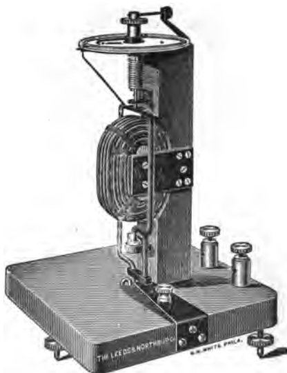
FIG. 2,519. —Leeds and Northrup electro-dynamometer. It is a reliable instrument for the measurement of alternating currents of commercial frequencies. When wound with fine wire and used in connection with properly wound resistances, it is equally useful for measuring alternating pressures, and may thus be employed to calibrate alternating current voltmeters as well as ammeters. To give accurate results the instruments must be carefully constructed and designed with a view to avoiding the eddy currents always set up by alternating currents in masses of metal near, or in the circuits. The constant of a dynamometer may be obtained with a potentiometer, but this is usually done with precision by the manufacturer and a certificate giving the value of the constant is furnished with the instrument. The size and cost of dynamometers rapidly increase with the maximum currents which they are designed to carry, and when more than 500 amperes are to be measured, the use of other instruments and methods is recommended.
