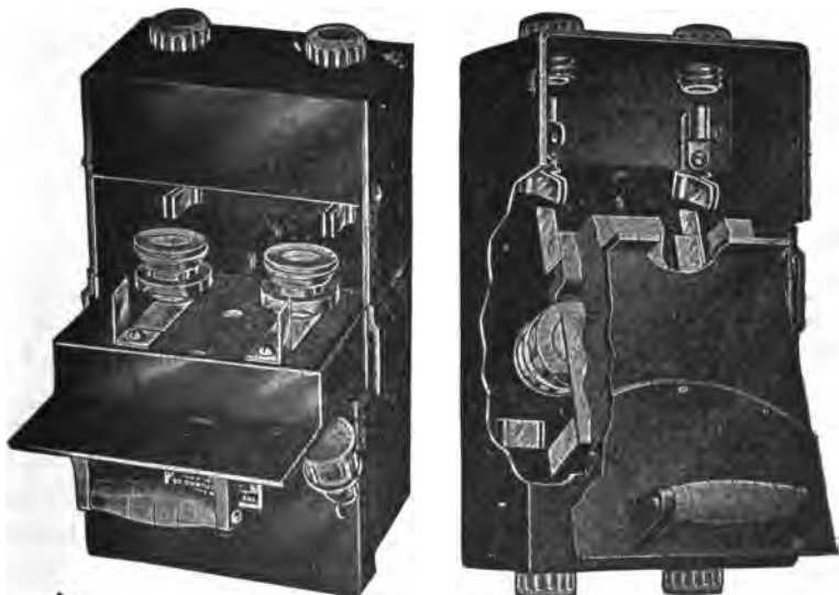
FIGS. 2,201 and 2,202. —Palmer service switch and fuse box, for either plug, cartridge or open link fuses. Fig. 2,201 illustrates the box in open position for the inspection of fuses, etc. The cover is held open by a simple lock so that the switch cannot fall closed by gravity, the box may be mounted so that the service wires lead directly into a sealed terminal chamber from any direction, and all current carrying parts made accessible by the opening of the switch are dead. Fig. 2,202 illustrates the device with side of box and cover cut away to show interior and the normally sealed cover of terminal chamber removed. The switch contacts do not enter their contact clips until the flanged cover of the box has closed the switch opening, no current connections being made to line or load until the box is completely closed, and in consequence there is no opportunity to make improper connections to any live parts of switch, when conduit connections are used to the service and meter wires.
