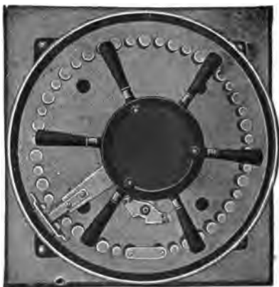
FIG. 2,435. —Dial of Westinghouse dial type variable ratio voltage regulator. The dial consists of a marble slab, upon which the contacts are mounted in a circle as shown. The contact arm is arranged to move from contact to contact. The alternate small contacts are dummies, serving to prevent the contact arm springing down between contacts when moving from one to another. The panel contains a changing switch which makes it possible to double the range of a regulator, since the transformer connections can be changed to both raise and lower to an extent equal to the full range of the transformer. The total range in voltage from a certain per cent. below to a certain per cent. above the line voltage can be obtained in a number of steps equal to twice the number of divisions into which the secondary winding of the transformer is divided.
