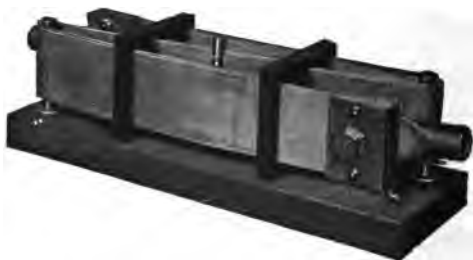
FIG. 2,423. —General Electric adjustable compensation shunt. It is used as the compensating shunt for direct current voltage regulators. In operation, the shunt may be adjusted so as to compensate for any desired line drop up to 15 per cent. It is preferably placed in the principal lighting feeder but may be connected to the bus bars so that it will take the total current. The latter method is sometimes undesirable, as large fluctuating power loads on separate feeders might disturb the regulation of the lighting feeders. Adjustment is made by sliding the movable contact shown at the center of the shunt. This contact may be clamped at any desired point and it determines the pressure across the compensating winding of the regulator's control magnet. Where pressure wires are run back to the central station from the center of distribution, they may be connected directly to the pressure winding of the main control magnet, and it is unnecessary to use the compensating shunt.
