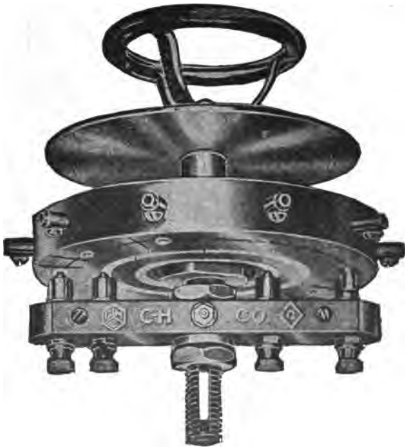
FIG. 2,648. —Crouse-Hinds voltmeter and ground detector radial switch, arranged for mounting on the switchboard. The switch proper is placed on the rear of the board with hand wheel, dial, and indicator only on the front side. The current carrying parts are of hard brass, with contact surfaces machined after assembling. The contact parts are of the plunger spring type, and the cross bar has fuse connections. Ground detector circuits are marked G+ and G- for two wire system, and G+, G-, GN+, and GN- for three wire system. When the voltmeter switch is to be used as a ground detector, two circuits are required for a two wire system, and four circuits for a three wire system, that is, a six circuit voltmeter and ground detector switch for use on a two wire system has two circuits for ground detector and four circuits for voltmeter readings. A six circuit voltmeter and ground detector switch, for use on a three wire system, has four circuits for ground detector and two circuits for voltmeter readings.
