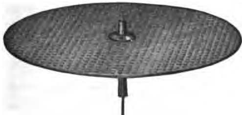
FIG. 2,547. —Moving element of Sangamo single phase induction watt hour meter. It consists of a light aluminum disc mounted on a hard brass shaft, the entire system weighing 15.6 grams. The disc is swaged under heavy pressure, to render it stiff. The arrangement of the disc, shaft, and bearings is shown in fig. 2,548. By unscrewing the upper and lower bearings the disc and shaft can be removed without disturbing the magnets or adjustments.
