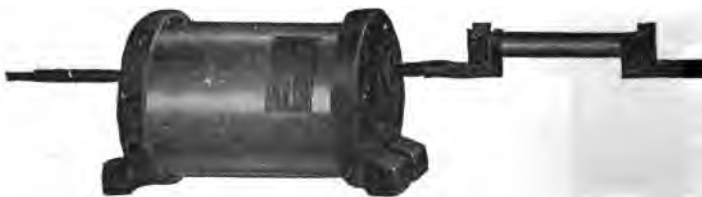
FIG. 2,405.—General Electric magnetic blow out arrester for line use. It consists essentially of a small spark gap which is in series with a resistance, and between the poles of a magnet. The operation is similar to that of the arrester shown in figs. 2,402 to 2,404, but the magnet is a permanent magnet instead of an electromagnet. The spark gap and the magnet are mounted within porcelain blocks in such a way that the discharge arc is blown by the magnet through an arc chute and a cooling grid which is also held by the porcelain. The cooling grid in the arc chute materially assists the magnet in extinguishing the discharge arc, giving the arrester a high arc rupturing quality. The series rod is carborundum and is connected externally to the other portion of the arrester. The arrester is self-contained.
