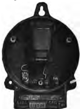
FIG. 2,551. —Base and shunt coil of Sangamo single phase induction watt hour meter. Since the shunt or pressure coil sometimes breaks down or burns out, due to abnormal line conditions or accident, provision is made for easy replacement. The shunt magnet with its coil is held to the base by two dowel pins and four screws, enabling it to be removed as a unit as shown. A new core and coil may then be substituted without the necessity of removing and replacing laminations. The shunt coil in 25 cycle meters is wider and contains more steel than the 60 and 133 cycle coils, the winding also being correspondingly increased. The return plate and series coil laminations are also changed in proportion to correspond to the increased width of the shunt magnet. The laminations forming the core are laced into the shunt coil, and subjected to enormous hydraulic pressure, the rivets being set at the same time, to form a compact unit and eliminate humming. The laminated core of the shunt element has but a single air gap in which these discs rotate.
