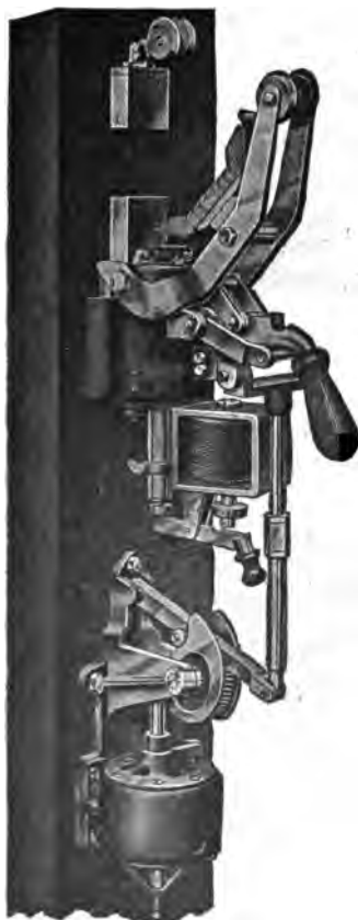
FIG. 2,304. —Condit 600 volt, 1,500 ampere single pole back connected type K circuit breaker, motor operated. The mechanical and electrical features of the circuit breakers are no different than when hand operated, the only difference being that the motor is used for the operating means. This motor is so arranged that even should it over travel, due to an accident to the controlling circuit, it cannot produce more than a pre-determined strain on the circuit breaker. In other words, after the motor has closed the circuit breaker, further travel of the motor will not result in putting a strain on the operating parts. Suitable motors are supplied for this service, the type of motor varying in accordance with the character of the operating current supplied. The advantage of this type of electrical operation is that it puts very little strain on the switch mechanism, takes very little operating current, allows the use of standard parts, and makes an extremely substantial and flexible structure. Its disadvantage is that it closes slowly, and it must not, therefore, be used in places where quick closing is essential.
