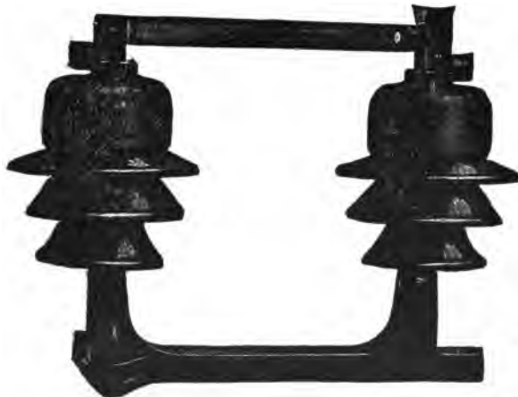
FIG. 2,208. —Westinghouse single pole disconnecting switch. Disconnecting switches are used primarily for isolating apparatus from the circuit for purposes of inspection and repair; also for sectionalizing feeders. They are not designed for opening under load, and therefore no attempt should be made to open them with current in the circuit. In connection with lightning arrester installations, disconnecting switches are particularly useful, providing a simple and effective means for isolating the arresters while cleaning and inspecting. The switch is opened and closed with a hook on the end of a wooden pole, which hook engages in a hole provided in the switch blade. This type of disconnecting switch is intended for wall mounting. The live parts are mounted on porcelain insulators carried on a cast iron yoke or base, forming a simple and substantial construction.
