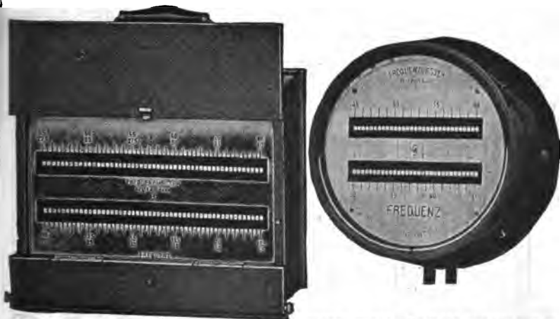
FIGS. 2,563 and 2,564.—Frahm resonance type frequency meter. Fig. 2,563, portable meter; fig. 2,564, switchboard meter. The readings are correct in either the vertical or horizontal position. The energy consumption at 100 volts is about 1 to 2 volt amperes, and is approximately proportional for other pressures. The regular portable meters are arranged for pressures of from 50 to 300 volts, and for this purpose they are fitted with terminals for 65, 100, 130, 180, and 250 volts. In order to obtain full amplitude at intermediate pressures, a milled headed screw is provided for adjusting the base piece mechanically, and thereby permitting of regulating the pressure range within \pm 20 per cent; this insures indications of maximum clearness. Should it be desired to extend the standard pressure range of 50 to 300 volts, up to 600 volts, two further terminals for 350 and 500 volts are necessary, so that these instruments are provided with eight fixed terminals in addition to the mechanical regulating device. Instruments which are intended for connecting to one specific supply or to the secondary of a pressure transformer, require only a single pressure range, say 100 volts, with the aforementioned regulating device. The frequency range is from 7.5 to 600 cycles per second. In order to obtain easily readable indications, one reed is provided for every quarter period for frequencies below 30, for every half period for frequencies between 30 and 80, and for every whole period for frequencies between 80 and 140. The use of a smaller number of reed, that is to say, of larger intervals between the periods of vibration of adjoining reeds, is only recommended for circuits having very variable frequencies, as otherwise no reed might respond to the vibrations caused by intermediate frequencies. The arrangement of the separate reeds on a common base piece, permits supplying any combination of interval that may be required. It is often desirable to secure two ranges with one set of reed. To do this a second electromagnet is supplied. It is polarized, and operates on the same base plate. In the case of alternating current when the unpolarized magnet is used the reeds receive two impulses during each cycle, while with the polarized magnet they receive but one impulse per cycle. A commutator is provided to easily make the change from one range to the other. If there be two sets of reed, the one commutator may be connected to change both. This device is only applicable when alternating current is measured. Instruments with unpolarized magnets are made with frequencies of 15 to 300 cycles per second.
