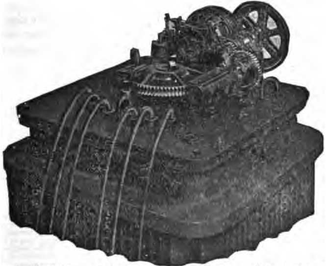
FIG. 2,422. —Westinghouse polyphase motor operated induction regulator showing operating mechanism. The primary shaft is turned by means of a bronze worm wheel engaging a forged steel worm, provided with a ball bearing end thrust. This worm gear is housed in a separate casting bolted to the cover. The casting is made separate in order to permit close adjustment between the worm wheel and the worm to aid in counteracting the tendency to vibration. Finished surfaces on the worm gear casting are provided for mounting the motor and the brake. On the automatic regulator, the worm shaft is connected to the motor through a spur gear and pinion, which constitutes a compact driving device having very little friction. Provision is made for either alternating current or direct current motor drive. When a motor driven regulator is operated by hand, the brake must be held in the release position, otherwise it will be impossible to operate the regulator. In the hand operated regulator the spur gear is replaced by a hand wheel and the regulator is driven directly from the worm shaft.
