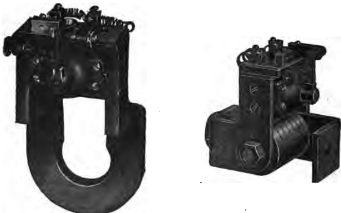
FIGS. 2,338 and 2,339. —General Electric instantaneous direct current reverse current or “discriminating” relays. Fig. 2,338, for 500 amperes; fig. 2,339 for 2,000 amperes. These relays are designed for mounting directly on circuit breaker studs. These relays consist of a horseshoe magnet with a shunt wound armature pivoted between its poles. The magnet is mounted on the current carrying stud of the circuit breaker between the back of the panel and the first contact or supporting nut, and is placed in a vertical position. The contacts are insulated from the magnet permitting the use of an auxiliary circuit for the tripping device, independent of the circuit controlled by the circuit breaker. The magnet is excited by the current flowing through the stud, and the armature is connected across the line in series with suitable resistance. Rotation of the armature in the normal direction is prevented by a stop. Reversal of the current flowing through the stud changes the direction in which the armature tends to rotate, causing it to move away from the stop and close the circuit through an auxiliary trip coil and trip the circuit breaker. These relays are used to protect dynamos, storage batteries, or main station busses from damage on reversal of current due to short circuit, or from the grounding of machines or connection. Relay contacts must not be used to open the shunt trip coil circuits. An auxiliary switch should be provided for this purpose in all cases where the opening of the circuit breaker does not disconnect the trip coil from the source of supply.
