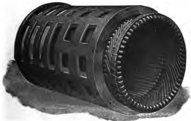
FIG. 2,420. —Bottom end of stationary element or secondary of Westinghouse polyphase induction regulator.
