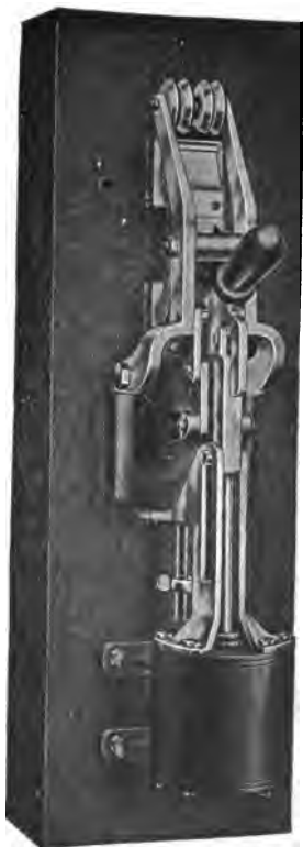
FIG. 2,331.—Condit 600 volt, 1,500 ampere, single pole type K circuit breaker pneumatically operated. It is the same as the electrically operated circuit breaker, except that a pneumatic cylinder mechanism is supplied in place of either the electromagnet or the motor. This cylinder mechanism is so arranged that the air pressure
