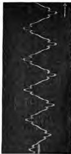
FIG. 2,635.—Short circuit current on direct current end of rotary converter, 21,500 amperes maximum. Upper curve, direct current voltage; lower curve, direct current amperage. Duration of short circuit about .1 second.
