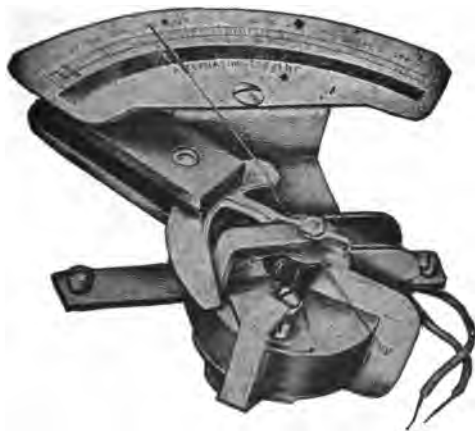
FIG. 2,512. —Hoskins instrument with case removed. It has a very short magnetic circuit which is composed of silicon steel, permitting low magnetic densities to be used.
