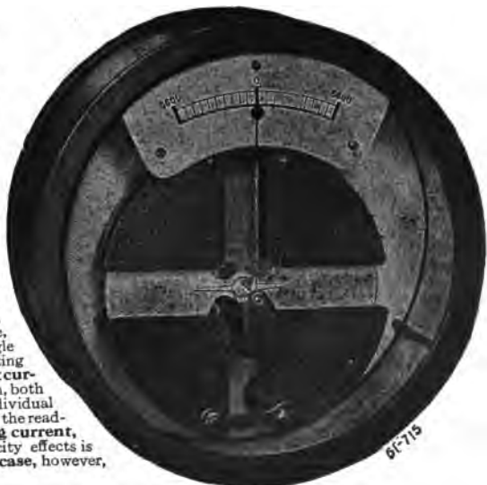
FIG. 2,580.—Westinghouse single phase electrostatic ground detector.
