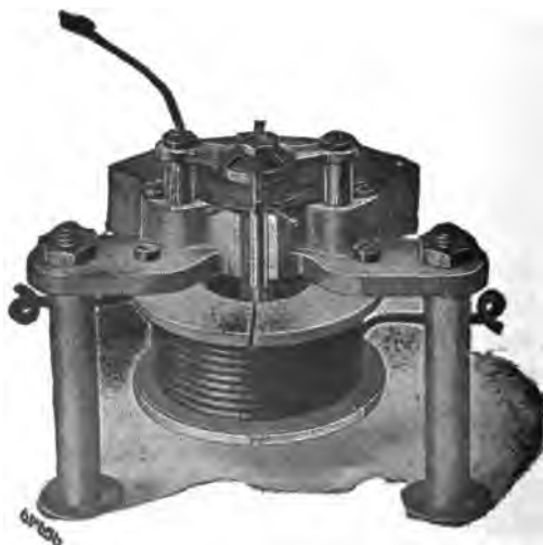
FIG. 2,500.—Magnetic vane movement of a Wagner instrument; it is used both for voltmeters and ammeters. This type differs from the dynamometer movement in that a vane of very soft iron replaces the moving coil. The magnetic vane movement makes use of its controlling spring only for the purpose of resisting the pull on the vane and the returning of the needle to zero. The spring does not carry any current. Digitized by Google
