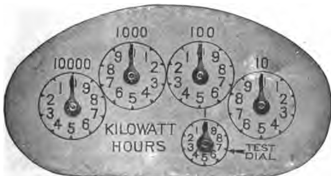
FIG. 2,550. —Canadian dial of Sangamo single phase induction watt hour meter. It has a small test circle indicating one kilowatt hour per revolution in all sizes where the first regular circle indicates 10. This is provided to conform with the requirements of the Canadian government and it is intended that the hand on the test circle shall make not less than \frac{1}{2} revolution in one hour with full load on a meter. In the case of a 10 ampere meter, it will make one complete revolution in one hour and for a 20 ampere, two revolutions, and so on. The train or indicating mechanism is carried on a rigidly formed and swaged brass bracket, accurately located by two dowel pins set in the top face of the main grid, and is held to the grid with two screws easily accessible when it is desired to remove the train for any purpose. All indicating trains used on type "H" meters are marked with symbols on the back of the train and on the compound attachment to indicate the gear ratio of each combination; this ratio being different for meters of different capacities in order to obtain a direct reading in kilowatt hours on the dial.
