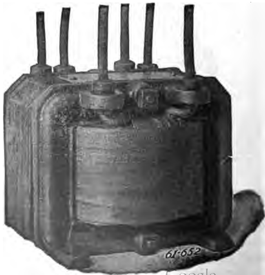
FIG. 2,516. — Wagner 25 watt pressure transformer for use with various alternating current instruments, such as voltmeters, wattmeters, etc. They are made in capacities 25, 50, 100, and 200 watts, and are built for pressures of 750 to 60,000 volts.
