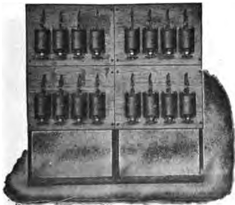
FIG. 2,453.—Westinghouse unit switch type pressure regulator, designed for handling heavy currents where a variable ratio transformer type of regulator is desired. The regulator consists of a number of electrically operated switches controlled from a master switch. These switches are arranged to perform practically the same cycle of operation as previously described for the drum type regulators. The transformer windings are divided into sections, and two floating coils are provided which are connected to various taps on the main auto-transformer. These floating coils have intermediate steps, and the successive operation of the switches connects the floating coils in proper sequence to the main auto-transformer, and transfers the line connection from one point of the floating coil to the next. In this way a 23 point regulator with sixteen switches, and a 71 point regulator with 21 switches may be supplied. The master switches are arranged with an automatic lock to prevent their being operated too rapidly. The magnet switches themselves are so interlocked that the proper sequence of operation is insured. The electrically operated switches may be of the open type, mounted on a slate or marble switchboard, when the whole control outfit is placed in a room which is comparatively free from dust or dirt of any kind, and where there is no danger of employees coming in contact with the switches. The other type of switch is entirely enclosed, the main contacts being oil immersed. The frames of these switches are grounded and the whole design is arranged to operate under ordinary dirty conditions. All of these switches, however, should receive the necessary inspection and attention. The contacts have a long life and are easily renewed. Regulators of this type are adapted for metallurgical purposes where the regulation is effected in the primary circuit and the secondary circuit is of very low voltage but large current capacity and is used for supplying power to the furnaces. These regulators have been built in capacities up to 800 amperes at 3,300 volts.
