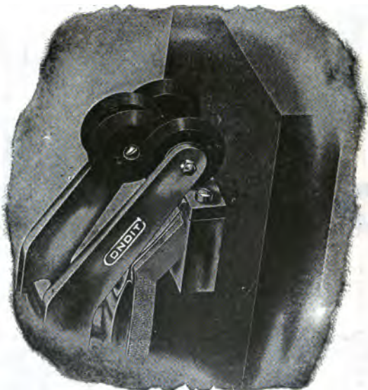
FIG. 2248. —Carbon break discs of Condit circuit breaker. The two pairs of similar discs which slide past each other are so arranged that these surfaces coincide at the instant the intermediate contact separates after which, as the contact arm opens further, they gradually disengage.
