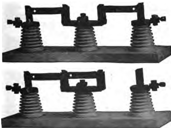
FIGS. 2,211 and 2,212.—Westinghouse selector type disconnecting switch. Fig. 2,211, view showing both sides closed; fig. 2,212, view with one side open. The selector type of disconnecting switch is a transfer switch which does not require the circuit to be interrupted while making the change. It can also be used to connect two independent circuits in parallel. In construction, it is in effect two single throw, single pole disconnecting switches with the hinge jaws connected together and mounted on the same insulator. The hinge jaw is also provided with dummy jaws to hold either blade of the switch in the open position. Except for these differences in the hinge jaws, the construction is similar to the switch shown in fig. 2,209. It should not be used to open the circuit when loaded.
