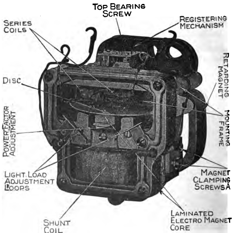
FIG. 2.528.—Westinghouse single phase induction type watt hour meter removed from case.
