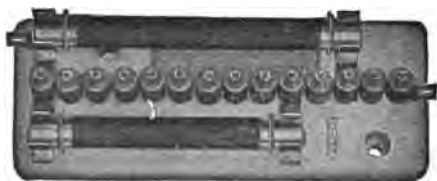
FIG. 2,351. —General Electric 2,200 volt multi-gap arrester for station installation. It consists of fourteen \frac{5}{8} " knurled cylinders and two shunt resistance rods mounted on a pre-cast base. One of these rods has a low resistance, and shunts nine gaps; the other rod has a high resistance, and shunts eleven gaps. The effect of the shunt resistance in extinguishing the line current arc is the same, therefore, as that of an equal series resistance but is without the objectionable features of the latter. Series resistance limits the discharge current to such an extent that an arrester with series resistance fails to protect against destructive rises of voltage when the conditions are severest. Graded shunt resistance responds to all frequencies and opens a discharge path for excessive voltage when the frequencies are high as well as when they are low. Its further effect is in withholding the line current from the gaps after the relieving discharge has occurred, is to aid the non-arcing quality of the metal cylinders in quickly suppressing the arc that follows a discharge. The arc is extinguished at the end of the half cycle of line current in which the discharge takes place.
