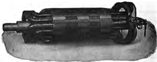
FIG. 2,417. —Moving element or primary of Westinghouse motor operated single phase induction regulator. It consists of a core of punchings built up directly on the primary shaft and carrying the primary winding, which is divided into four coils. The primary coils are machine wound and the layers of the winding are separated from each other by heavy insulating material in addition to the cotton covering of the inductors. The complete coils are insulated and impregnated with insulating compound before being placed in the slots. The coils are held in position by fibre wedges.
