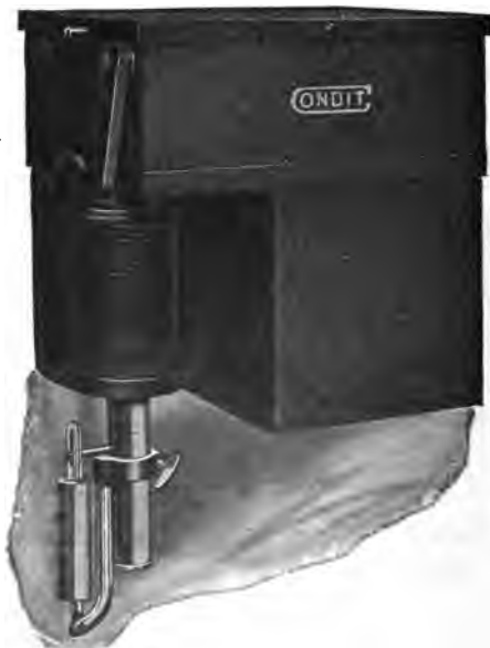
FIG. 2.310. —Condit type "B" time limit attachment, designed to give sufficient time to allow an induction motor to start without opening the circuit breaker, and not have the circuit breaker trip on the momentary rush of current. Its action is inverse ; that is, the greater the current the less time it takes to operate and is so arranged that four to five times full load current or a short circuit will trip the circuit breaker instantly. The time limit attachment is applied directly to the armature which trips the circuit breaker and is adapted for the so called primary trip. It consists of an air vacuum dash pot with a graphite piston, the dash pot being fastened to the stationary calibrating ring of the trip coil and the moving outside cylinder is fastened to the armature of the circuit breaker. When the current reaches a point where it overcomes the weight of the armature and lifts the same, the magnetic force tending to raise the armature is opposed by the vacuum created in the interior of the cylinder. As the magnetic force continues, the vacuum is overcome due to the leakage of air past the plunger and the armature gradually moves up until it reaches the point where it trips the circuit breaker. If at any point of the armature travel, the current drop back to normal, the armature immediately resets itself by means of a ball valve in the top of the brass cylinder
