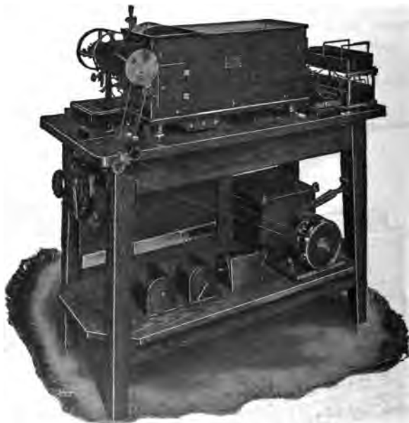
FIG. 2,599. —General Electric moving coil oscillograph complete with tracing table. The tracing table is employed for observing the waves, and by using a piece of transparent paper, the waves under observation appear as a continuous band of light which can be traced, thus making a permanent record. This is not, however, to be regarded as a recording attachment, and can not be used where instantaneous phenomena are being investigated. The synchronous motor for operating the synchronous mirror in connection with tracing and viewing attachment is wound for 100 to 115 volts, 25 to 125 cycles, and should, of course, be run from the same machine which furnishes power to the circuit under observation. A rheostat for steadying and adjusting the current should be connected in series with the motor. The beam from the vibrator mirrors striking this synchronous mirror moves back and forth over the curved glass, and gives the length of the wave; the movement of the vibrator mirror gives the amplitude, and the combination gives the wave complete. An arc lamp or projection lantern produces the image reflected by the mirrors upon the film, tracing table or screen. For the rotation of the photographic film, a small direct current shunt wound motor is ordinarily used.
