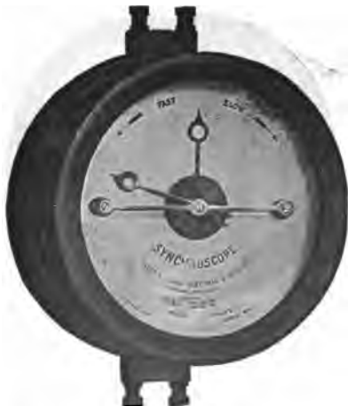
FIG. 2,570. —Westinghouse rotary type of synchroscope or synchronism indicator. The indication is by means of a pointer which assumes at every instant a position corresponding to the phase angle between the pressures of the busbars and the incoming machine, and therefore rotates when the incoming machine is not in synchronism. The direction of rotation indicates whether the machine be fast or slow, and the speed of rotation depends on the difference in frequency. The pointer is continuously visible, during both the dark and light periods of the synchronizing lamps.
