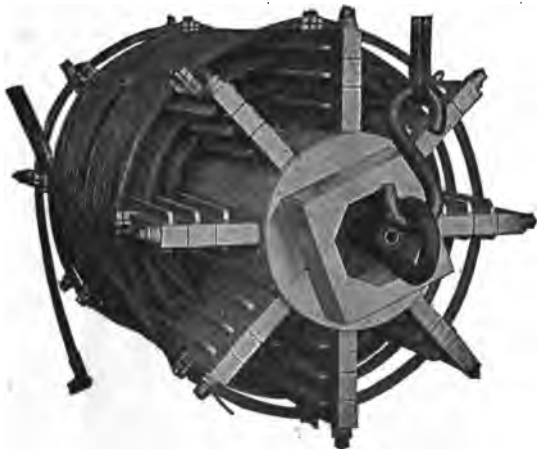
FIG. 2,243. —General Electric current limiting reactance; view showing details of construction. The core consists of a hollow concrete cylinder; alloy anchor plates or sockets being embedded in the core near the ends to receive the radial brass bolts. An extension at each end of the core provides for clamping and bracing the reactance in installation. The supports for the winding are made of resin treated maple and are located upon the core by radial brass studs screwed into the alloy sockets, and insulated by mica tubes. The nuts by which the structure is tightened, rest upon heavy fibre washers. Wooden barriers fitted and shellaced into the supports add to the creepage surface between layers of the winding and between the winding and the core. The supports of the layer next to the core are separated from the core by strips of treated pressboard. The coil consists of bare stranded cable in several layers, usually three in number. It is wound into grooves in the treated wood supports, which are protected from contact with the cable by heat shields of asbestos shellaced into the grooves. The winding is usually in the form of two back turn sections, thereby allowing the terminals of the coil to be brought out at the ends of the outside layer. This assures accessibility and ease of connection, and the removal of the leads from proximity to the core. Two turns at each end of the winding are given extra spacing for the purpose of additional insulation. The final turn at each end of the coil is securely held in place by alloy clamps bolted to the supports. The wood is protected from contact with the clamps by shields of asbestos. The ends of the cable between the two sections are welded by the oxy-acetylene process.
