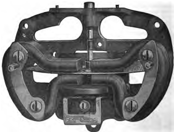
FIG. 2,546. —Main grid or supporting frame of Sangamo single phase induction watt hour meter. The grid is of cast iron and its design is such that the weight of the permanent magnets, series laminated element and return plate are carried on the main portion, the smaller projecting brackets carrying no weight except that of the moving system. The supporting grid is removed by taking out the three screws locating and holding it in position, to the iron base, also removing at the same time the screws connecting the leads of the series coils to the binding posts at the bottom. The meters are all built with four binding posts so that they may be connected either with two series leads and a tap for the pressure connection or with both sides of the circuit carried through the meter. The wire meters employ a 220 volt shunt coil, connected across the binding posts within the meter, one series coil being in each of the outer lines of the three wire system. This renders unnecessary the use of a pressure tap.
