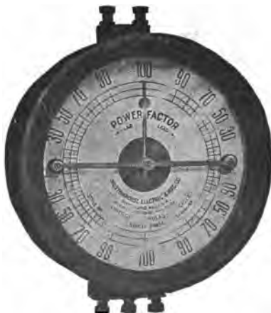
FIG. 2,578.—Westinghouse rotating field type power factor meter. The rotating field is produced by the currents of the metered circuits in angularly placed coils, one for each phase of the system, in the case of polyphase meters. In the three phase meter the rotating field is produced by three coils spaced 60^\circ apart; in the two phase meter by two coils spaced 90^\circ ; in the single phase meter the positions of voltage and current coils are interchanged and the rotating field is produced by means of a split phase winding, connected to the voltage circuit. There are no movable coils or flexible connections. Single phase meters indicate the power factor of a single phase circuit, or of one branch of any polyphase circuit. Special calibration is necessary in order to use a single phase instrument on a three phase circuit unless the voltage coil be connected from one line to the neutral. Polyphase meters indicate the average angle between the currents and voltages and are superior for polyphase service to meters having only one current coil.
