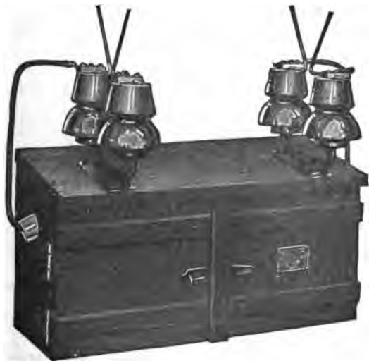
FIG. 2,382.—General Electric horn arrester for pole installation. Quite frequently series circuits are run underground in cables for some distance from the generating station. In order to protect the cables it is advisable to place horn arresters at the points where the cable joins the overhead wires. The resistance units are mounted in the wooden box. This design is used to economize space, since if the horn gaps be placed in the box the latter would have to be made very large to accommodate the asbestos barriers and backs. In installing this type of arrester it is advisable to place it as near as possible to the top of the pole so that the arc may rise unobstructed and thus avoid the likelihood of live wires coming in contact with the horns which, during the operation of the series current, are alive.
