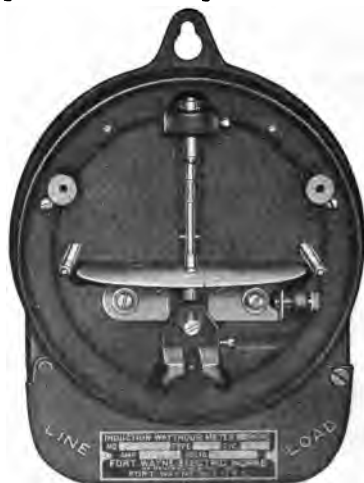
FIG. 2,544. —Fort Wayne single phase induction watt-hour meter with cover register and permanent magnets removed to show solid meter frame. A heavy steel back plate held in place by two screws inserted from the front of the central casting encloses the back part of the completely assembled meter. A felt gasket lying on a suitable ledge seals the joint against the entrance of dust or moisture when the back plate is drawn down firmly by the screws. The cover which encloses the back part of the meter is a non-magnetic metallic stamping. It is held in place by wing nuts on the two light brass studs extending forward from the meter frame. This joint between the main frame and the cover is also sealed against the entrance of dust and moisture by the use of a suitable felt gasket. Two glass windows are provided in this cover, one to permit the reading of the register dials, the other to permit observation of the disc's rotation. The cover is sealed in place in the usual way by passing a sealing wire through a hole drilled in the cover sealing stud and thence through a hole provided in the wing of the seal nut. The terminal chamber is an extension of the casting which supports all the inner parts of the meter. The heavy brass terminals used for connecting the meter in circuit are held permanently by a non-combustible insulating compound which is moulded in place around them. This construction gives excellent insulation and is a safeguard against accidental short circuits across terminals. A punched terminal cover which fits over the terminal chamber is hinged at the upper left hand corner so that it will of its own accord swing out of the way when the terminal cover sealing screw is removed. This hinged style of cover will be found convenient when installing and connecting the meter in circuit. When this cover is swung back into closed position it is fastened in place by passing a seal right through the seal screw and through a lug provided on the cover.
