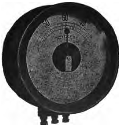
FIG. 2,567. —Westinghouse induction type frequency meter. The normal frequency is usually at the top of the scale to facilitate reading. The damping disc moves in a magnetic field, thus damping by the method of eddy currents. The standard meters are designed for circuits of 100 volts nominal and can be used for voltages up to 125 volts. For higher voltages, transformers with nominal 100 volt secondary should be used.
