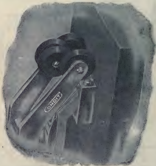
FIG. 2,248.—Carbon break discs of Condit circuit breaker. The two pairs of similar discs which slide past each other are so arranged that these surfaces coincide at the instant the intermediate contact separate after which, as the contact arm opens further, they gradually disengage.
