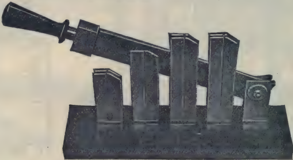
FIG. 2,218. —Westinghouse rear connected motor starting switch, for pressures up to 600 volts. It is used for starting rotary converters and direct current motors of large capacity having starting torque small enough to permit cutting out the starting resistance in few steps. The clips can be connected to any type of resistor, the steps of which are successively short circuited as the switch closes; the amount of resistance in the armature circuit is thus gradually reduced. A pause should be made after each step of resistance is thrown in to allow the motor speed to accelerate. If the starting switch do not have to carry the full load current and can be short circuited by another switch, a starting switch of smaller capacity equivalent to 50 per cent of running current of the machine can be used. The switch is of the single pole, single throw, rear connected, four point, knife blade type.
