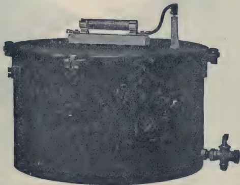
FIG. 2,398.—Westinghouse electrolytic station lightning arrester for direct current up to 1,500 volts consists of a tank of oil in which are placed, on properly insulated supports, a nest of cup shaped aluminum trays. The spaces between the trays are filled with electrolyte, a sufficient quantity for one charge being furnished with each arrester. The top tray is connected with the line through a 60 ampere fuse, and the bottom tray is connected to the tank which is thoroughly grounded by means of a lug. The fuse is of the enclosed type and mounted on the cover of the arrester. A small charging current flows through the trays continuously and keeps the films on the trays built up, so that no charging is required. This charging current is not, however, of sufficient value to raise the temperature appreciably. The immersed area of each tray is 100 square inches. The shape and the arrangement of the trays is such that any gases generated by the discharge can pass out readily without disturbing the electrolyte between the trays.
