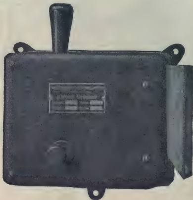
FIG. 2,244. —Westinghouse magnetic blow out circuit breaker, designed for the protection of street railway and electric locomotive equipments; it serves the combined purpose of fuse block and canopy switch. The contact tips are surrounded by a moulded arc chute which confines and directs the arc until the magnetic blow out extinguishes it. The current carrying contacts consist of copper strips separated by air spaces. An auxiliary contact or "arcing tip" at the end of the switch lever takes the burning of the arc when the breaker opens, and thus confines the burning to a very small piece which can be easily removed and replaced at small cost. The hand tripping lever and the resetting lever have insulated handles, so that they can be safely handled, even in the dark.
