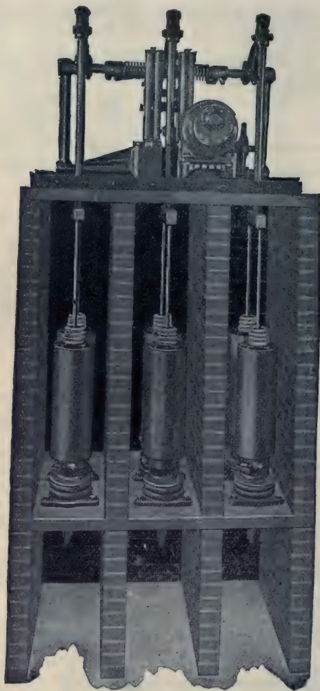
FIG. 2,232.—General Electric motor operated three phase oil switch. The operation of the oil switch is accomplished by a small hand controlling switch, generally mounted on the panel, with the instruments which are in the circuit controlled by the oil switch. The standard pressure for the operating motor is 125 volts. The switch has six breaks, each break being in a separate tank. In addition to this isolation of the breaks, each phase is enclosed in a fireproof brick compartment, making it impossible for trouble in one phase to be communicated to another. The cells are constructed of brick with top and bottom slabs of slate. The capacities of such switches, range from 2,500 to 60,000 volts, and from 100 to 1,000 amperes.
