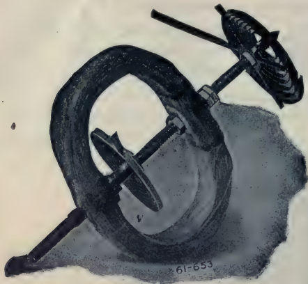
FIG. 2,515.—Armature of Wagner dynamometer movement. Greater accuracy is claimed for this movement than the magnetic vane, but it cannot readily be employed for the indication of current flow, as required in ammeters. The magnetic vane movement is used on the A. C. ammeter, and can be used also in the A. C. voltmeters; it makes use of its controlling spring only for the purpose of resisting the pull on the vane and the returning of the pointer to zero. The dynamometer movement is recommended for voltmeters.
