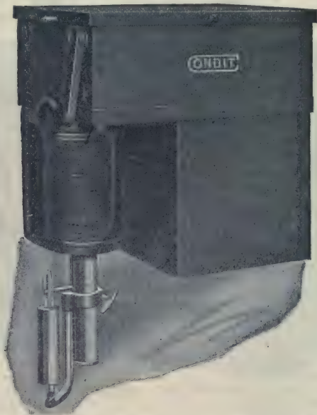
FIG. 2,310. —Condit type "B" time limit attachment, designed to give sufficient time to allow an induction motor to start without opening the circuit breaker, and not have the circuit breaker trip on the momentary rush of current. Its action is inverse; that is, the greater the current the less time it takes to operate and is so arranged that four to five times full load current or a short circuit will trip the circuit breaker instantly. The time limit attachment is applied directly to the armature which trips the circuit breaker and is adapted for the so called primary trip. It consists of an air vacuum dash pot with a graphite piston, the dash pot being fastened to the stationary calibrating ring of the trip coil and the moving outside cylinder is fastened to the armature of the circuit breaker. When the current reaches a point where it overcomes the weight of the armature and lifts the same, the magnetic force tending to raise the armature is opposed by the vacuum created in the interior of the cylinder. As the magnetic force continues, the vacuum is overcome due to the leakage of air past the plunger and the armature gradually moves up until it reaches the point where it trips the circuit breaker. If at any point of the armature travel, the current drop back to normal, the armature immediately resets itself by means of a ball valve in the top of the brass cylinder
