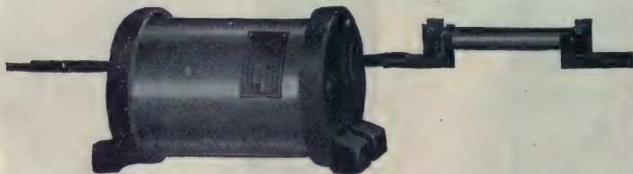
FIG. 2,405.—General Electric magnetic blow out arrester for line use. It consists essentially of a small spark gap which is in series with a resistance, and between the poles of a magnet. The operation is similar to that of the arrester shown in figs. 2,402 to 2,404, but the magnet is a permanent magnet instead of an electromagnet. The spark gap and the magnet are mounted within porcelain blocks in such a way that the discharge arc is blown by the magnet through an arc chute and a cooling grid which is also held by the porcelain. The cooling grid in the arc chute materially assists the magnet in extinguishing the discharge arc, giving the arrester a high arc rupturing quality. The series rod is carborundum and is connected externally to the other portion of the arrester. The arrester is self-contained.
