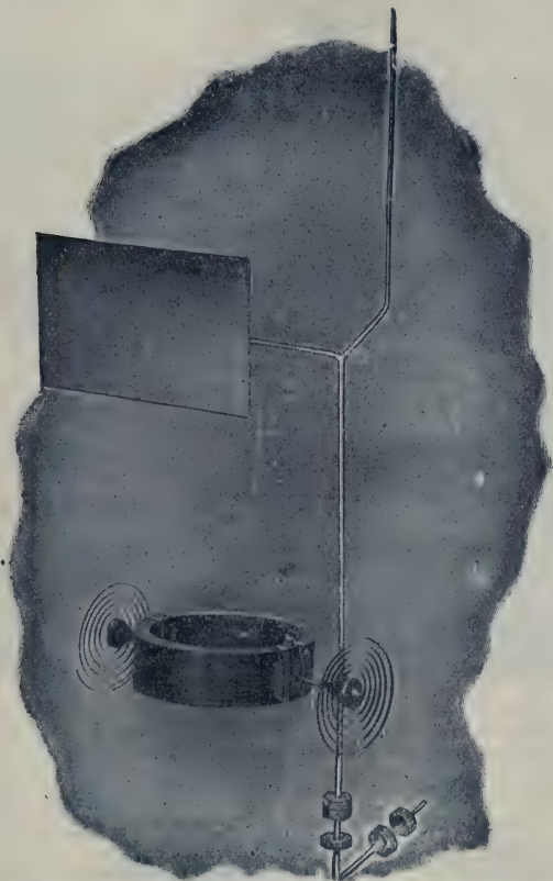
FIG. 2,517. —Moving element of Keystone dynamometer instrument. The illustration shows the movable coil, pointer, aluminum air vane for damping the oscillations, controlling springs, and counter weights.
