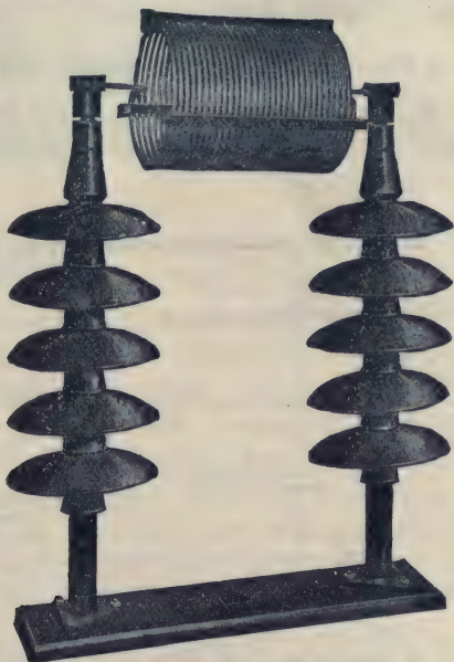
FIG. 2,412.—Westinghouse air cooled choke coil, for voltages of from 2,200 to 110,000. In construction , the coils are made of aluminum rod wound into a helix of about 15 inches in diameter and having 20 turns. The helix is supported on two insulators. For mechanical reasons it is necessary to have the aluminum rod of sufficient size to secure rigidity, consequently every coil has a capacity of 200 amperes and may be used on any circuit up to that capacity. The coils are insulated according to the standard practice for disconnecting switches, the insulators being mounted on wooden pins supported by a wooden base. This apparatus can be mounted in any position. The wiring of a station or sub-station is facilitated because the protection may be placed so as to simply form part of the wiring. The coils are symmetrical so that it is immaterial which end is connected to the line or to the apparatus.
