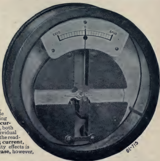
FIG. 2,580.—Westinghouse single phase electrostatic ground detector.
