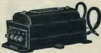
FIG. 3,308.—Western Electric bell ringing transformer. A self contained unit for use on 60 cycle alternating circuit of 100-125 volts. Delivers current at 6, 12, or 18 volts.
