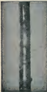
FIGS. 3,438 to 3,440.—Behavior of tantalum filament. Fig. 3,438, unburned tantalum filament; fig. 3,439 tantalum filament after burning 800 hours on alternating current; fig. 3,440, tantalum filament after burning 800 hours on alternating current. The new filament is smooth and without regular structure, while after burning for some time, it begins to take on a crystalline appearance. This change takes place less rapidly with direct than with alternating current, so that the life of the lamp is somewhat greater in the former case. When the filament finally burns out, it is supposed to be due to the change from the amorphous to the crystalline state, as indicated in the illustrations.
