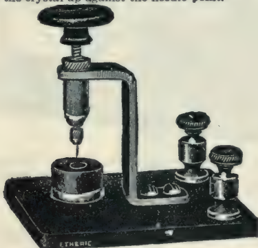
FIG. 3,170.—Electrolytic detector invented by Fessenden. It is probably the most sensitive of all detectors excepting the audion and the valve detectors. It consists of a carbon cup connected to a binding post and an adjustable standard which holds a very small hair-like platinum wire which dips into a 20% diluted solution of nitric acid. The high resistance of this acid detector is somewhat reduced by incoming wireless waves and when a telephone is shunted around it, the varying resistance is sufficient to vibrate the diaphragm but not strong enough to work a telegraph relay. When a potentiometer and battery are connected with the electrolytic detector and telephone, the sensitiveness is increased. The electrolytic detector is capable of operation with about three hundred micro-ergs; the magnetic detector is capable of operation with about four hundred micro-ergs; the silicon and most crystal detectors with about one thousand micro-ergs, and the manufactured carborundum detector with about nine thousand micro-ergs. Notwithstanding this very considerable difference in the sensitiveness of the electrolytic and carborundum detectors as measured by the C. G. S. system of units, in the actual practice of wireless telegraphy the receptive difference is hardly perceptible over similar distances. A great deal depends upon the adjustment of the detector which is a "cut and try" procedure until the most sensitive point is arrived at which will best respond to incoming signals.
