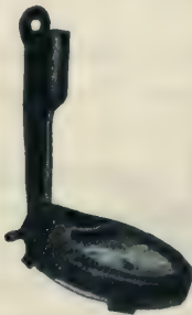
FIG. 3,540. —Adams-Bagnall clutch as used on series arc lamp. The clutch proper is of porcelain, and is placed loosely in a steel container, which is connected to the walking beam by means of an adjustable hook of substantial design. To prevent the carbon jarring through the clutch, the dash pot plunger is mounted by means of the stem directly on the clutch retainer. This produces a pinching effect on the carbon. The carbon, however, is readily released from this grip when the feeding point is reached.
