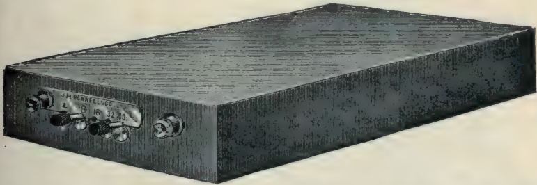
FIG. 3,081. —Bunnell adjustable telegraphic condenser showing 4, 8, 16, 32, and 40 per cent. peg adjustment. The interior construction consists of a number of sheet of tin foil interleaved with insulation, usually mica. As connected in the duplex system alternate leaves are connected with the artificial line and the intervening leaves to ground.
