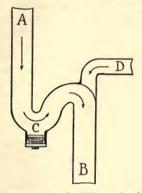
might force sewage back into the bowl. It has been believed that the vent does away with any possible siphoning or emptying of traps because of the sudden rush of water through them.
