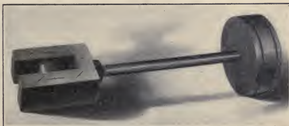
FIG. 68.—Piston, piston rod and crosshead.
