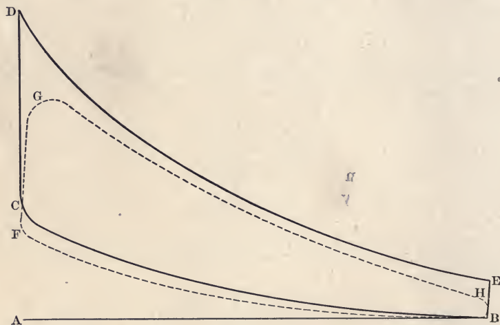
FIG. 172.—Difference between actual and theoretical indicator cards.
