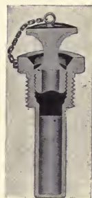
FIG. 8.—Portable Thermometer-cup. Sectional View.
