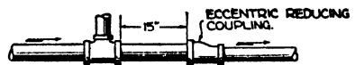
FIG. 5. METHOD OF CHANGING SIZE OF STEAM MAIN WHEN RUNOUTS ARE TAKEN FROM TOP
