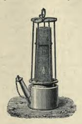
whose meshes are not too wide, over the flame of a Bunsen lamp, the flame is arrested by the gauze, although the un-
