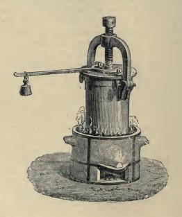
used for extracting everything soluble from bones, etc., is simply a very strong boiler, in which water, under the pressure of its saturated vapour, can be safely raised to temperatures far above its ordinary boiling-point.
