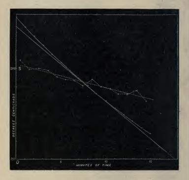
the thermometer after the lapse of successive intervals, equal or not, be plotted (on mechanically ruled paper) as above; intervals of time being measured horizontally, corresponding temperatures vertically. The figure represents, on a much
