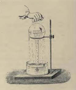
atmosphere (or, more accurately, to 9.16 millimetres of mercury). And a notable feature of this experiment is that the water is found to become gradually *colder* as the boiling proceeds, thus requiring farther exhaustion by the air-pump
