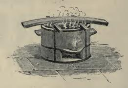
When a rod, or preferably a flat strip, of wood or metal is bent it is known that the layers on the convex side are
