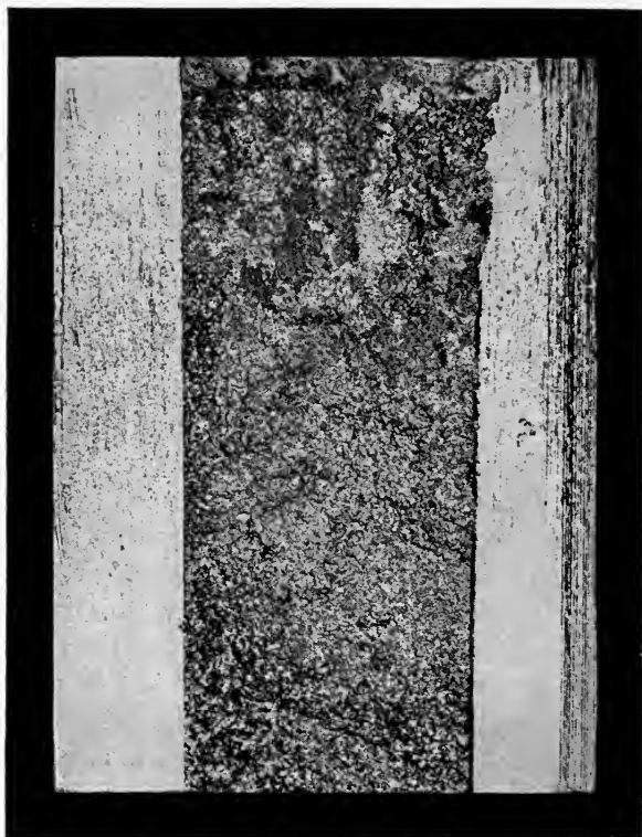
FIG. 8.—Effect of charcoal in dozzle.
