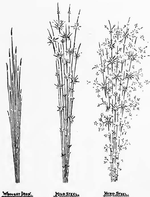
FIG. 73.—How sparks vary as carbon increases.
