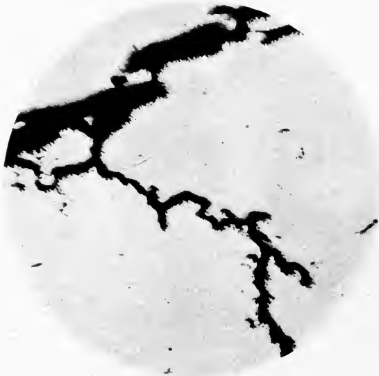
FIG. 43.—Forked crack following cementite outline (magnified 100 diameters).
