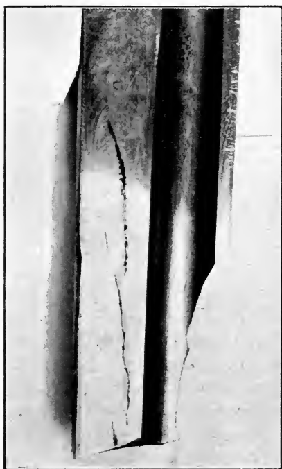
FIG. 46.—Crack on bevelled edge of sword-blade.
