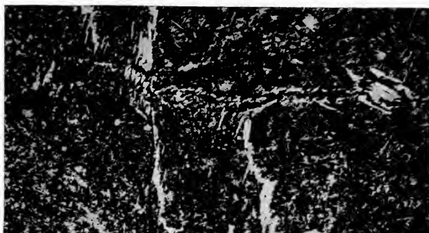
FIG. 14.—Crack following free cementite outline.
