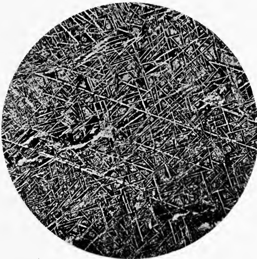
FIG. 7.—Free cementite needles in case-hardened steel. Photos at 100 diameters.
