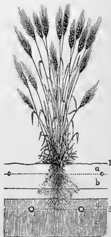
SECTION OF LAND AFTER IT IS DRAINED.
