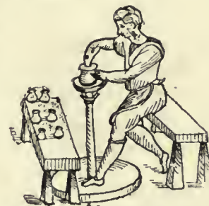
Fig. 4. From a Venetian wood cut of the middle of the 16th century; shows Majorica potter at work throwing pots on the wheel. The potter works his wheel by means of the lower foot-turned disk.
