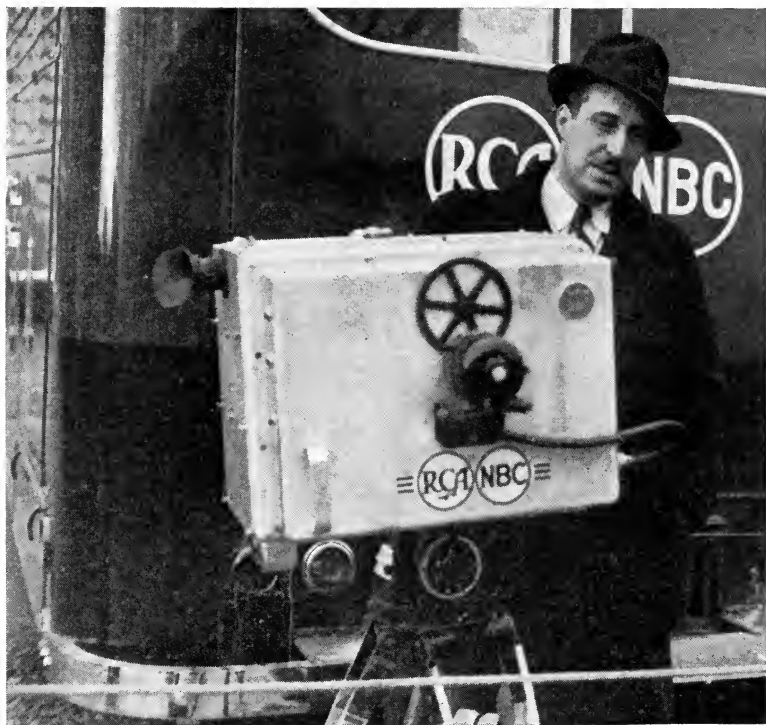
Remote control focusing device on mobile unit camera.
