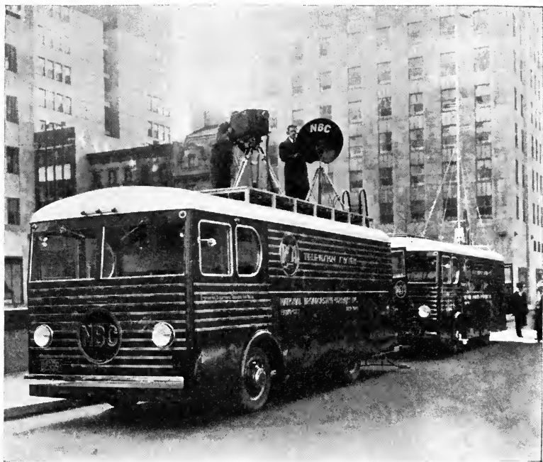
The mobile unit trucks in Rockefeller Plaza. The camera and parabolic microphone are being operated from the roof of the truck housing the control room. The antenna of the television relay transmitter on top of transmitter truck at right.
