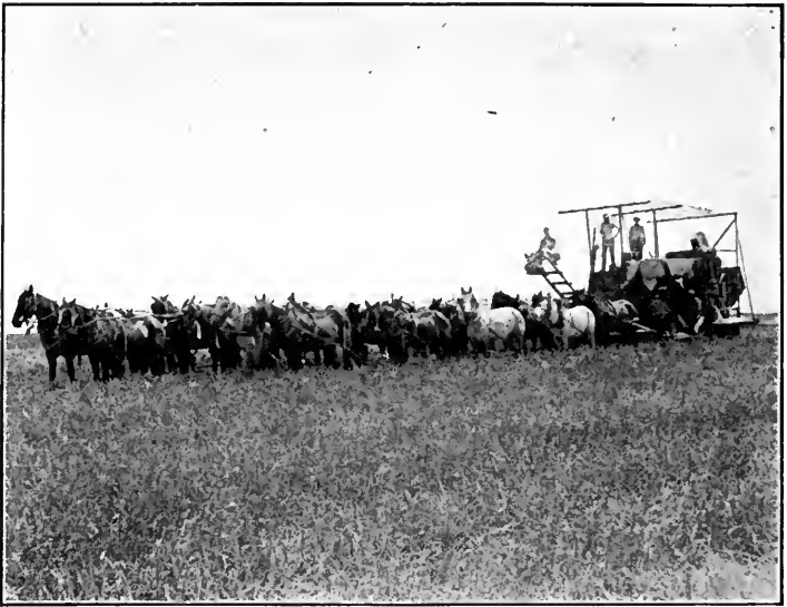
COMBINED HARVESTER AND THRASHER ON RANCH OF H. M. KINNEY, IMPERIAL VALLEY.
