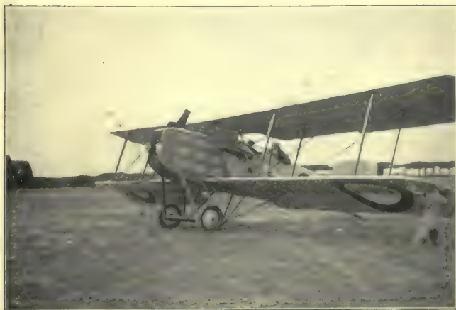
BREGUET TWO-PASSENGER BOMBING PLANE
