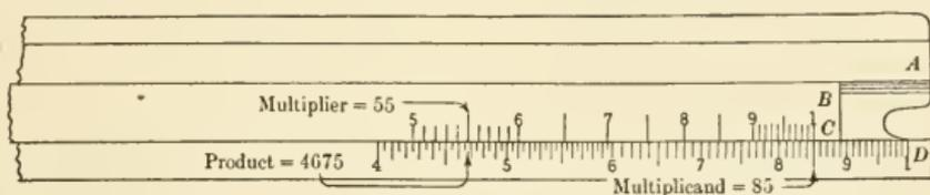
If we set the unit on *C* over 55 on *D*, or over 85 on *D*, the 85 on *C* or 55 on *C* will be off the *D*-scale to the right. This means that the two mantissas together are equal to more than a unit, and the characteristic of the logarithm of the product will be  $(1+1)+1$  carried from the mantissas. It is thus apparent that there will be four integral places in the result, and we place the decimal point accordingly.
