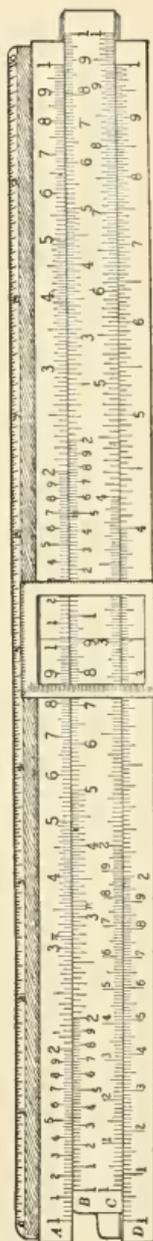
**Operations with the Slide Rule.** If we wish to multiply 2 by 2 on the slide rule we simply set 1 on the scale marked *C* exactly over 2 (the multiplicand) on the scale marked *D*, and under 2 (the multiplier) on *C* we read 4 (the product) on *D*.
