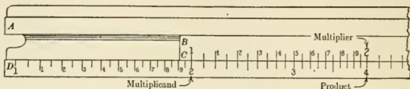
Similarly, to multiply 45 by 6, we set 1 on *C* over 45 on *D*, and under 6 on *C* we read 270 on *D*. In the case of decimals it is usually evident where to place the decimal point.
