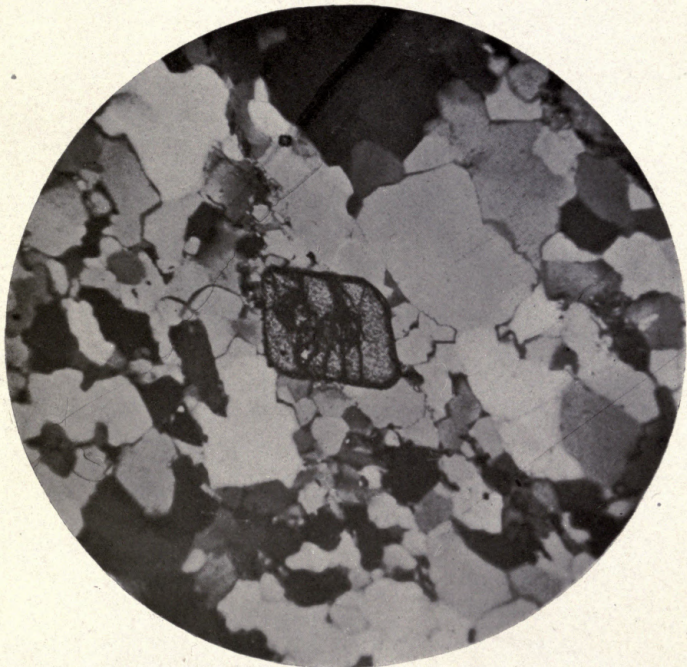
Fig. 3 Poughquag quartzite, Peekskill area; taken in polarized light (nicols crossed), magnification 65 diameters. The quartz grains are fairly free from included matter, and are firmly interlocked; the large crystal near the center of the field is a zircon of unusual size. No trace of the original rounded grains remains because of the complete reorganization of the rock.
