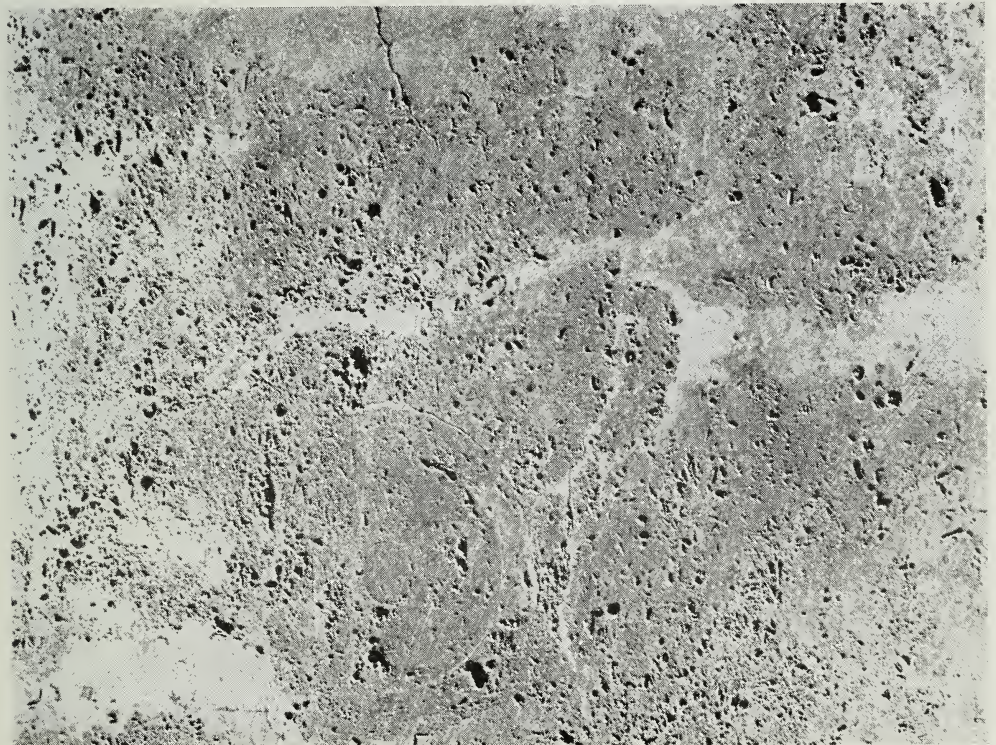
FIG. 3.—Smoothed surface of high-purity dolomite showing the porous texture. The dark areas are pores. (Natural size.)
