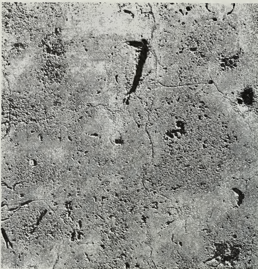
FIG. 33.—Smooth surface of Galena dolomite showing variations in porosity. The dark areas are holes or pores. (One-half natural size.)
