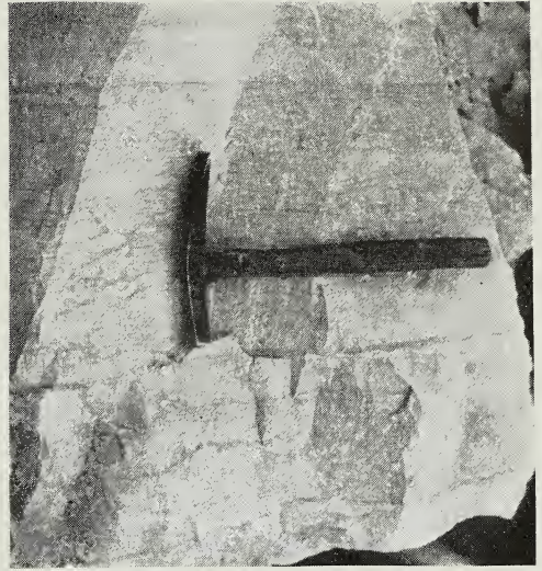
FIG. 2.—Dolomite containing clay partings and small nodules of white chert. The clay partings appear as thin dark wavy lines. Many are discontinuous.
