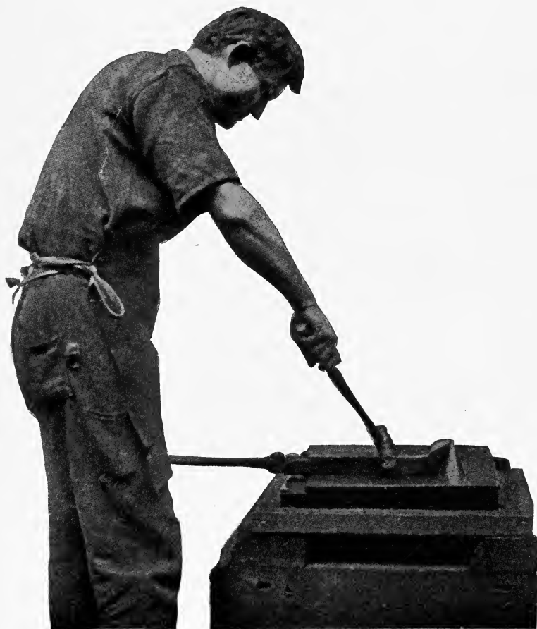
FIG. 56. Trying tool against cone gage to test proper angle for nose.
