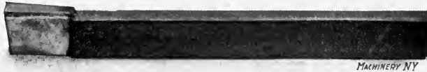
Fig. 149. A planer roughing tool with stock made of machinery steel and cutting edge of a relatively thin strip of high-speed steel brazed to the supporting stock. In use regularly in shops of the Lodge Shipley Machine Tool Company.
