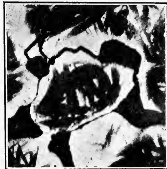
FIG. 11. Microscopic structure of high-speed steel ingot as cast. \times 1,000 .
