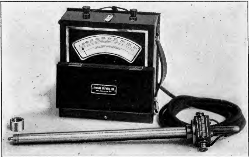
FIG. 126. Thermo-couple pyrometer enclosed in steel tube, and indicating instrument.
