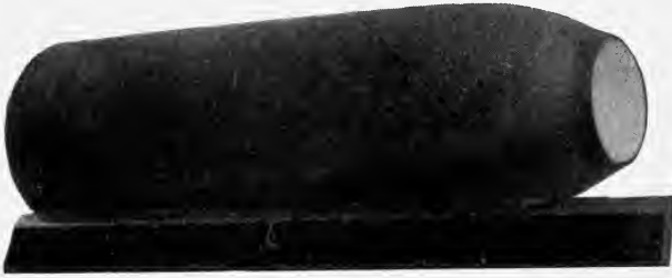
FIG. 166. Die for drawing down lead covering over table.
