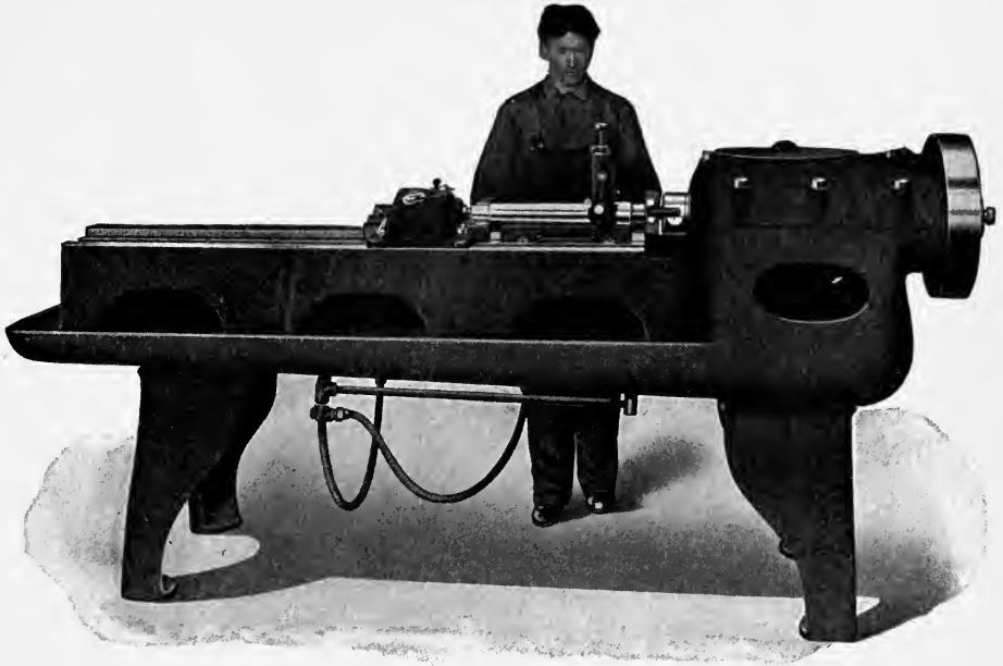
FIG. 243. "Lo-Swing" lathe (rear view) of the Fitchburg Machine Works. Unique design of bed — and indeed of machine throughout.
