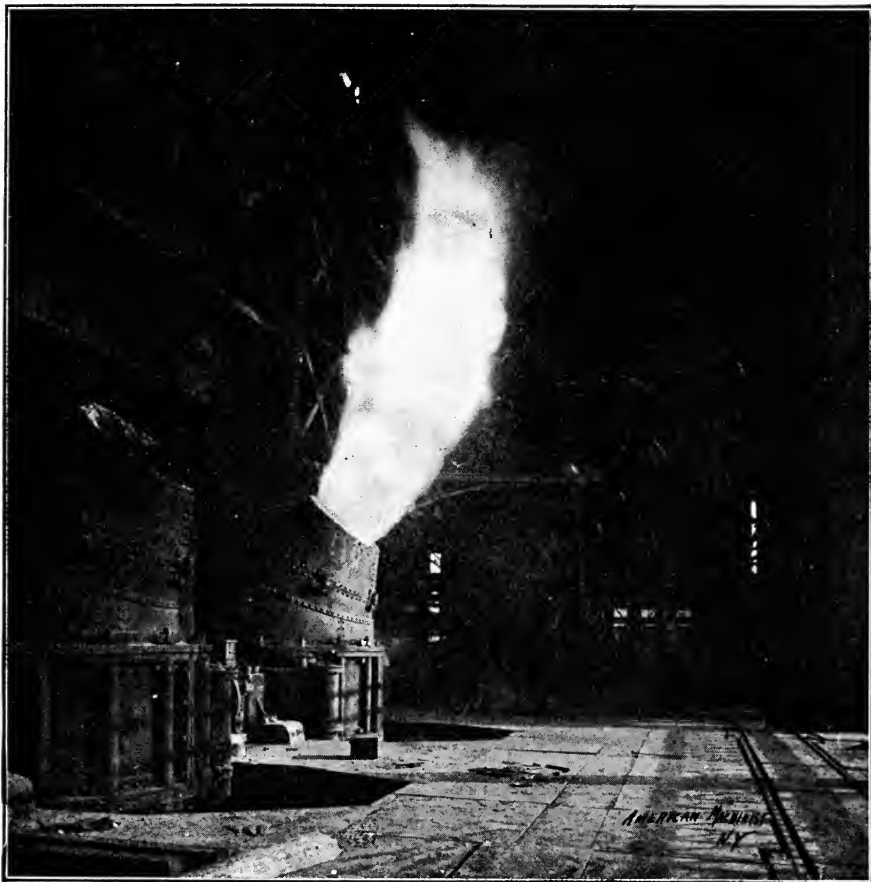
FIG. 6. The bessemer converter in action.
