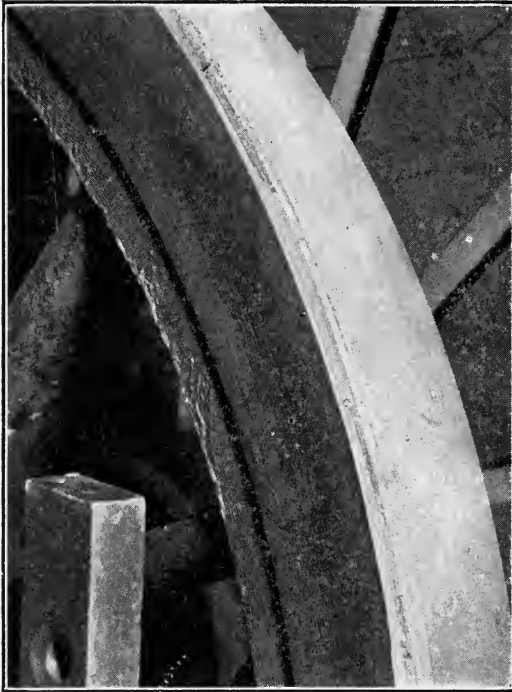
FIG. 171. Tread of locomotive tire after finishing. Note corrugations indicating vibration of tool.
