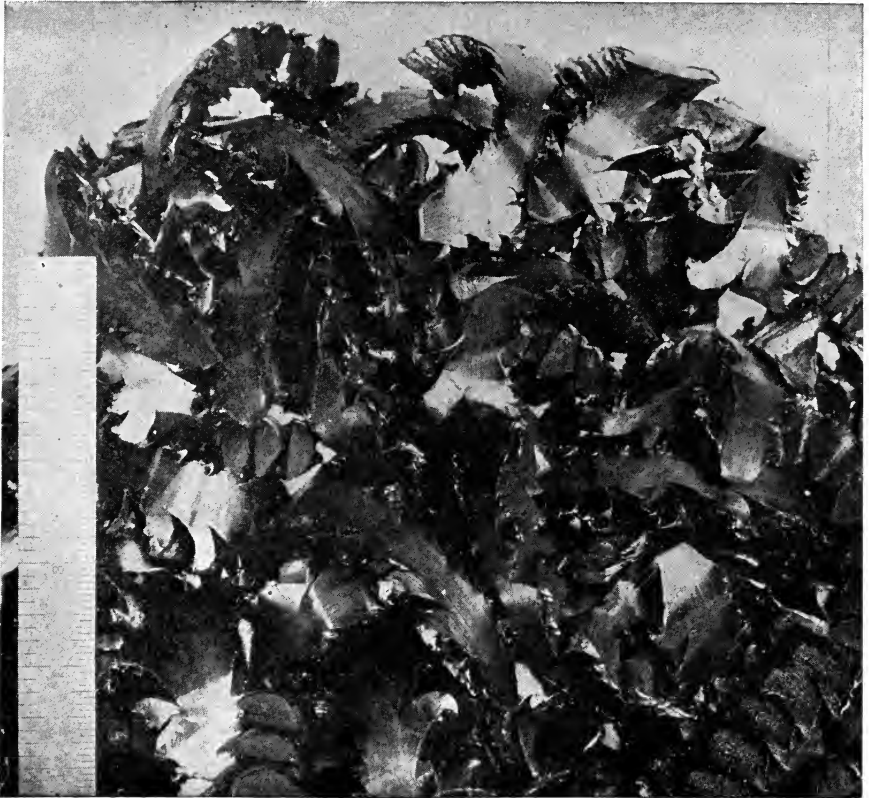
FIG. 152. The new steels are especially effective in heavy cutting. Chips even larger than these are by no means rare in certain shops.
