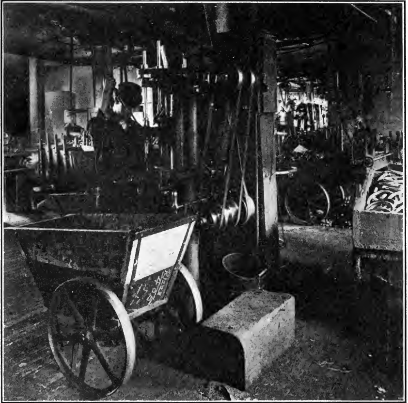
FIG. 267. Auxiliary storage by hand trucks. Very well if trucks are designed to fit the conditions and do not occupy an amount of space not permissible.
