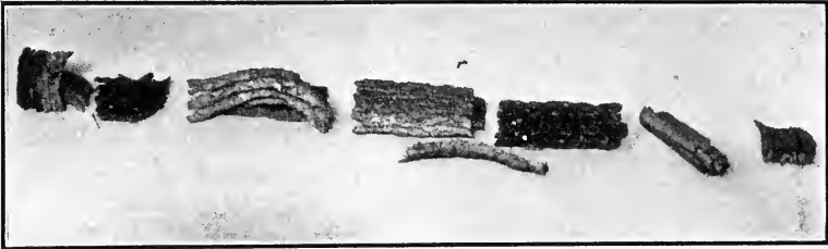
FIG. 184. Typical chips made in cutting cast iron.
