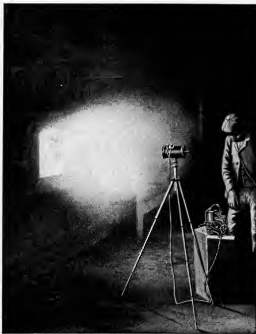
FIG. 140. Féry radiation pyrometer in use.
