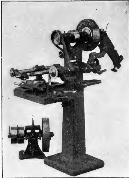
FIG. 106. Wilmarth & Mormon Company yankee drill grinder, with attachment for universal grinding. Very desirable in a small shop with a considerable range of tool grinding work.
