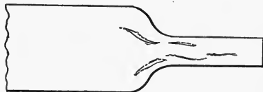
FIG. 48. What is likely to take place when the interior of a tool being forged is much hotter than the exterior.
