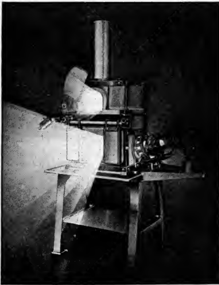
FIG. 61. Brayshaw twin-chambered hardening furnace, for oil or gas fuel. The illustration shows the furnace equipped for burning oil. The upper chamber is heated by waste heat from the lower, and is used for preheating.
