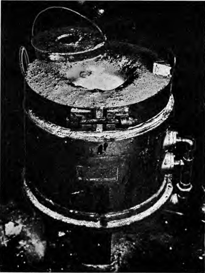
FIG. 80. A cylindrical gas furnace fitted for use with the barium chloride process. Crucible filled with melted salts and ready for use.
