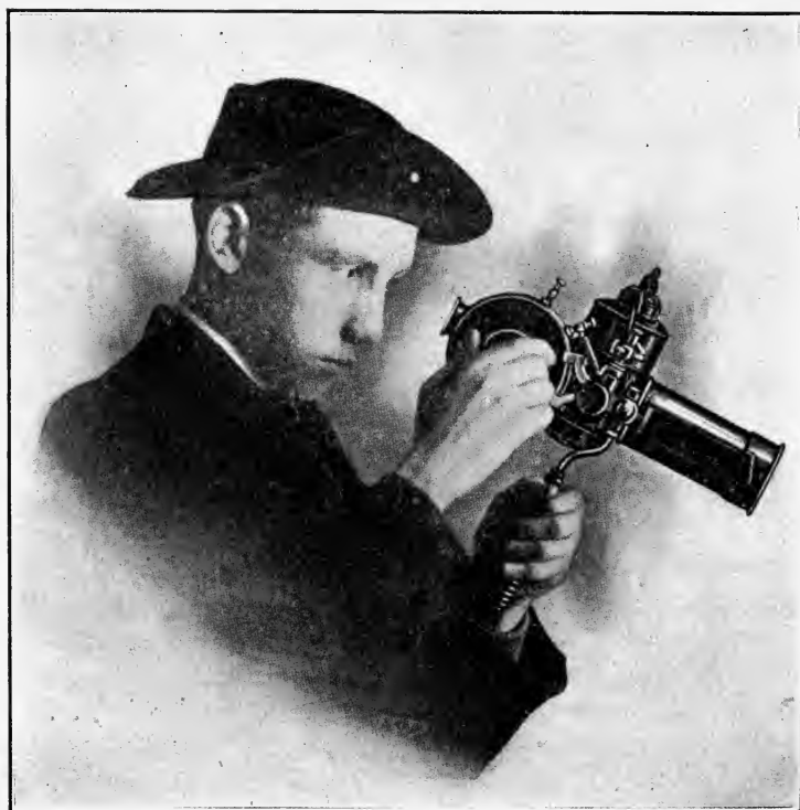
FIG. 138. The Morse Thermo Gage in use. It may also be used in connection with a portable stand.
