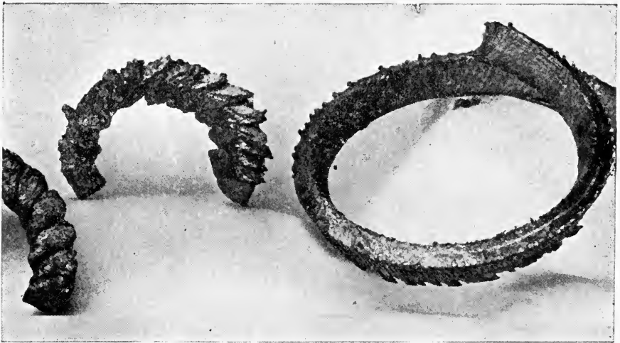
FIG. 216. Characteristic chips. Those at the left were made by a diamond point tool having 70 degrees cutting angle. Chips at the right made by a no-clearance tool, 45 degrees cutting angle. From "Machine Building for Profit," by James Hartness.
