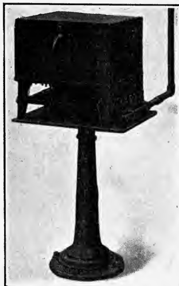
FIG. 93. A tempering plate with sheet-metal hood or oven, as used in the Crossly Brothers Motor Works.
