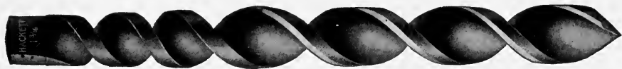
FIG. 236. Twisted drill made from a flat bar of stock throughout its entire length. Shank ground to standard taper.
