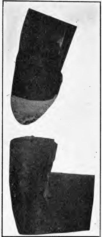
FIG. 183. Small particles of the chips scraped from the forging and pressed into a compact pile upon the lip surface of the tool.
