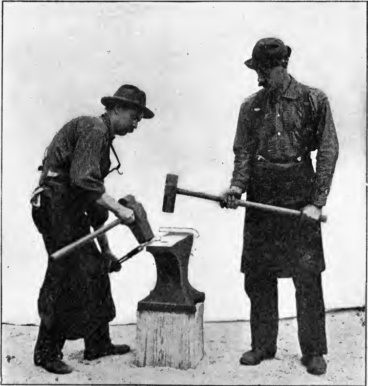
FIG. 53. Forming a side roughing tool.
