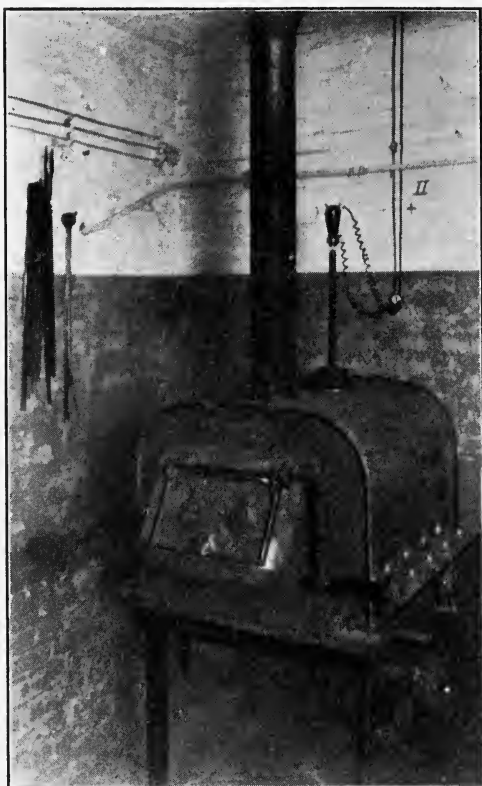
FIG. 123. Le Chatelier fire end inserted in oven furnace. The indicator is at any convenient distance.
