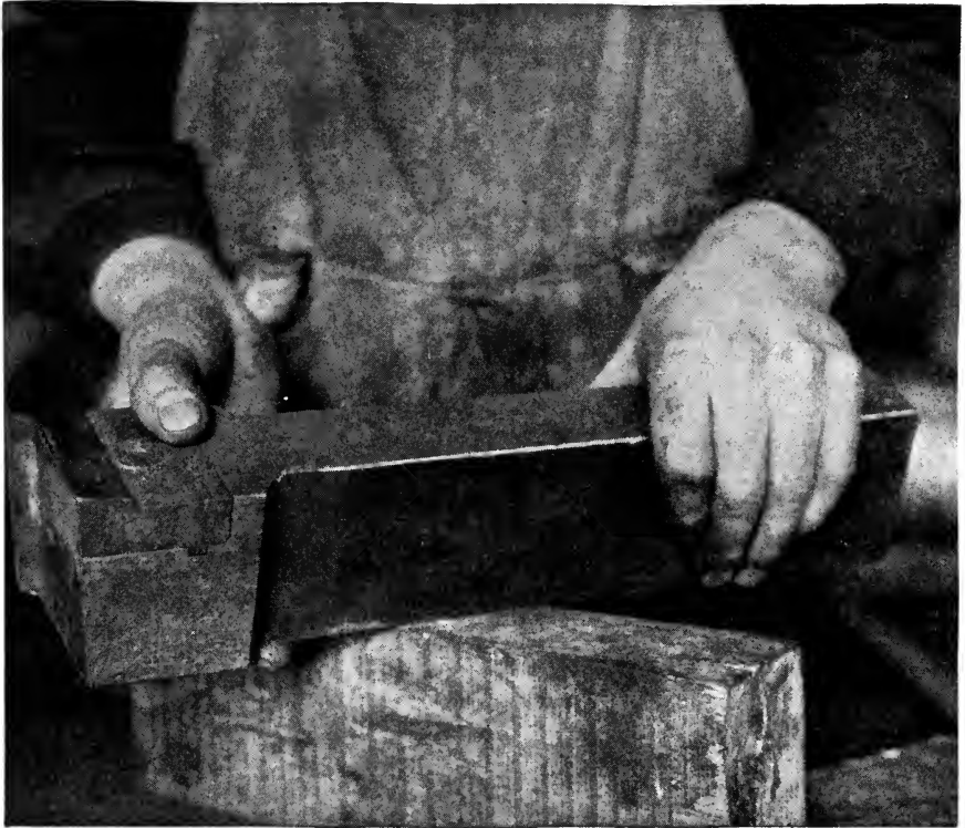
FIG. 220. A type of composite tool, suited to scraping.
