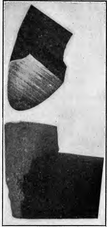
FIG. 187. Wear on tool run at proper speed. Tool still in good condition.
