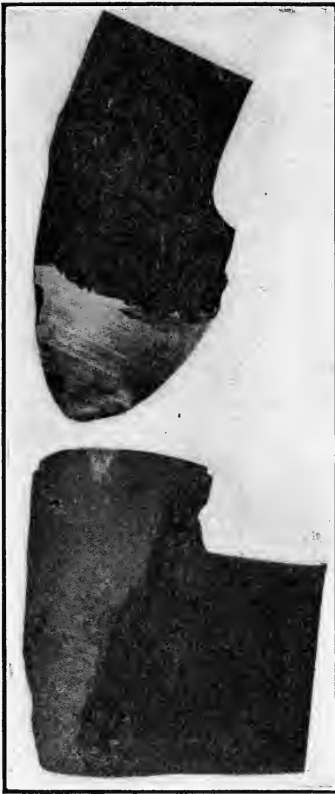
FIG. 186. Tool run at such high speed as to be ruined while cutting.
