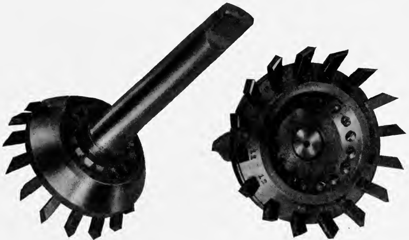
FIG. 223. An interesting composite milling cutter. So designed that the blades are easily removed and ground simultaneously by the aid of a grinding fixture. Courtesy of Mr. William G. Thumm.
