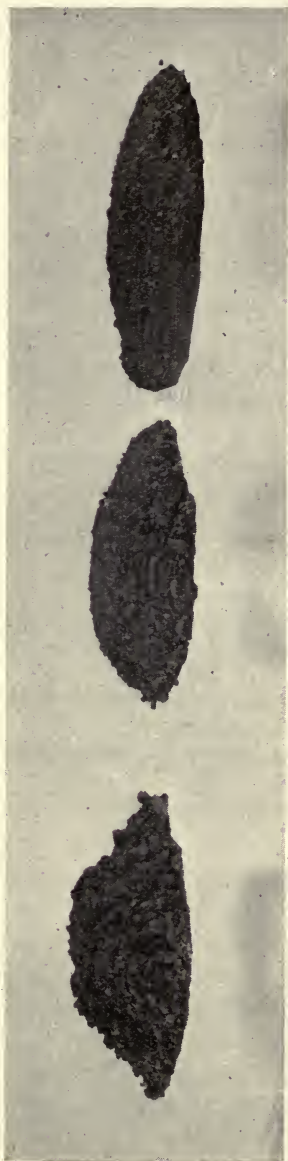
Fluid. Mushy. Quaking. FIG. 142.—Consistency of Concrete, Courtesy of U. S. Bureau of Standards.
