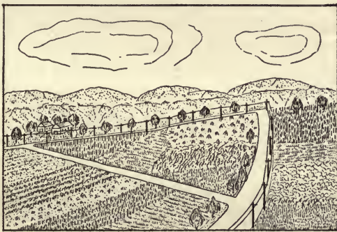
FIG. 12.—Frequently a Road May be Shortened and Two Hills and a Sharp Angle Eliminated by Cutting across a Corner
