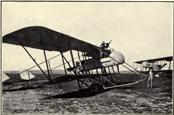
At the French aviation field, two miles from Belgrade. Eighty horsepower motor biplane. Capacity, two passengers. Plane has glass floor, carries five large bombs, five cans of flashettes, and other accessories. Aviator is cleaning and adjusting the Hotchkiss rapid-fire gun, preparatory to making a flight.
