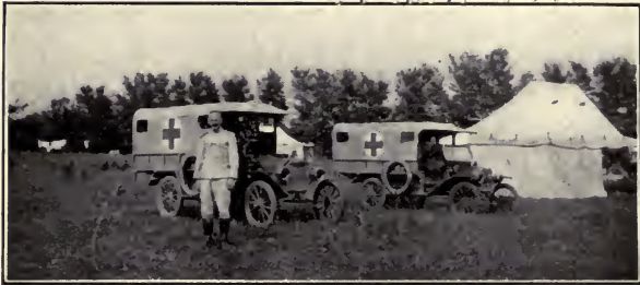
Ford ambulance, a very fine type of light, speedy ambulance that can negotiate the roughest roads. Capable of carrying four, recumbent. Used by the St. John's Ambulance Co. of Great Britain.
