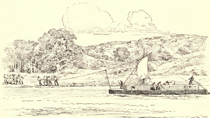
KEEL BOAT WITH CORDELLE, SAIL, AND POLES
