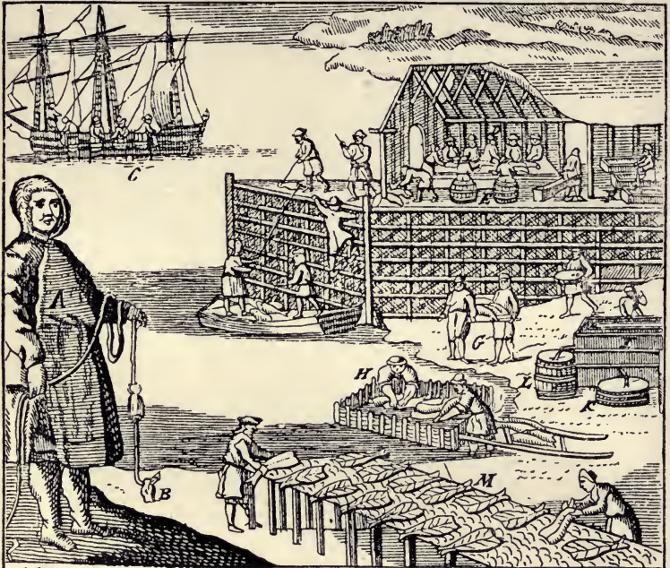
A View of a Stage, also of manner of Fishing for, Curing & Drying of Cod at NEW FOUND LAND. A. The Habit of the Fishermen. B. The Line. C. The manner of Fishing. D. The Dressers of the Fish. E. The Trough into which they throw the Cod when dressed. F. Salt Boxes. G. The manner of carrying the Cod. H. The Cleansing of the Cod. I. A Press to extract the Oyl from the Livers. K. A Cask to receive the Water and Blood that comes from the Livers. L. another Cask to receive the Oyl. M. The manner of drying the Cod.
