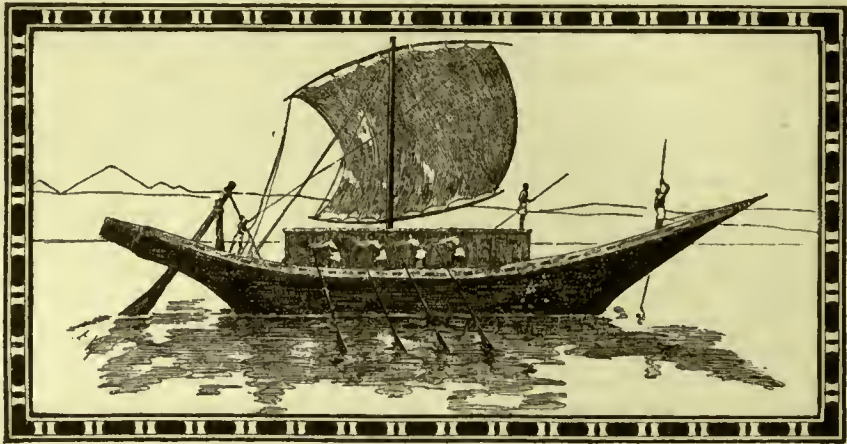
ANCIENT EGYPTIAN BOAT, SHOWING THE METHOD OF USING RUDDER, SAIL, AND OARS
