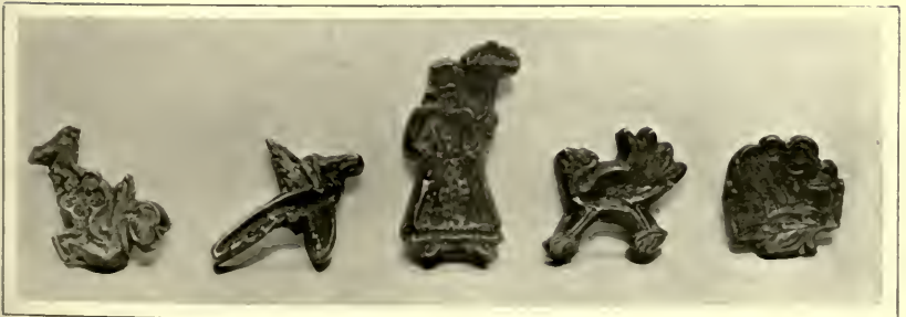
FIG. 11A —BRASS STAMPS, INCLUDING TWO OF THOSE USED FOR STAMPING THE ORNAMENTS ON ABOVE JUG.
