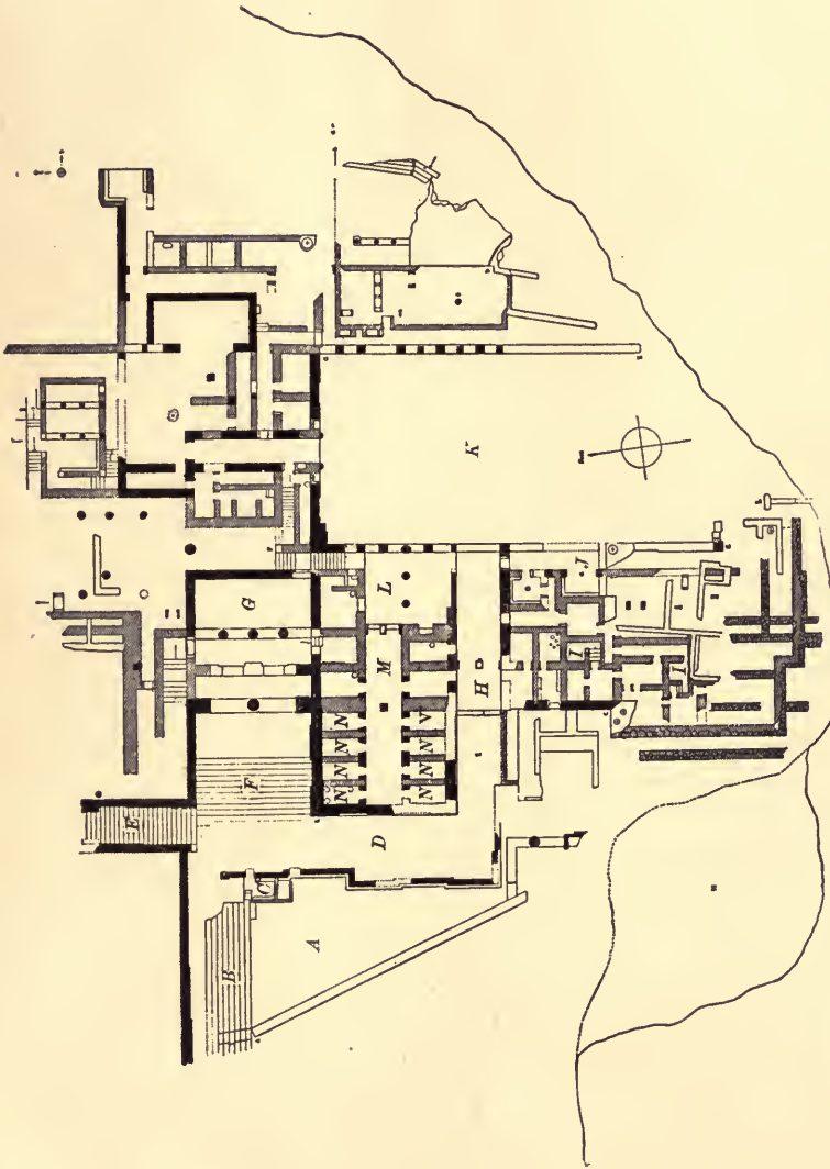
FIG. 205. — Plan of the palace at Phaestus. A , paved area. B , seats facing agora. C , altar. D , west corridor. E , staircase to upper story. F , staircase to upper hall. G , upper hall. H , megaron of men. I , interior corridor. J , bath-rooms. K , room with triglyph supports. L , central court. M , interior corridor. N , V , magazines.
