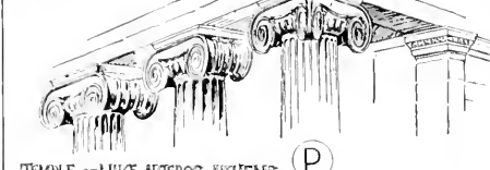
P TEMPLE OF NIKE-APTEROS ATHENS. SHELVING TREATMENT OF ANGLE CAP X ANTA. SKETCHED FROM A PHOTOGRAPH.
