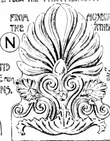
N ANTETRIX ORNAMENT TO COVER JOINT OF TILES ALONG EAVE OF ROOF.
