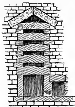
FIG. 2.—SECTION OF KING'S CHAMBER.
