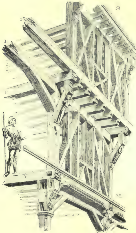
148—Timber ossature of a French house of the thirteenth century. (From Viollet-le-Duc.)
