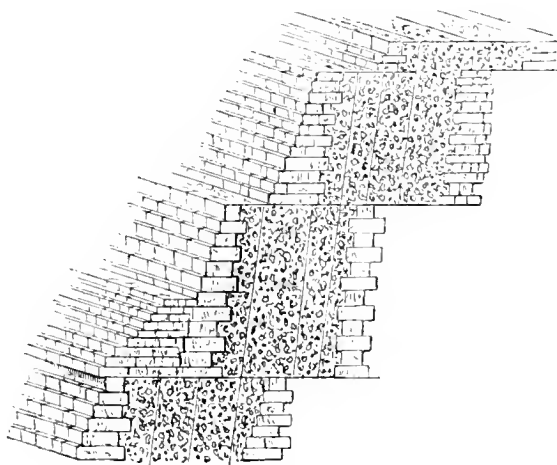
FIG. 144.—Construction of the Pyramid of Abousir in parallel layers ; transverse section in perspective from the geometrical section of Lepsius. 3
