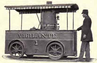
STEAM INSPECTION CAR.
