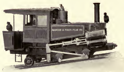
RACK LOCOMOTIVE, ABT SYSTEM.
