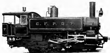
RACK LOCOMOTIVE, WITH TWO COG-WHEELS.
