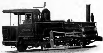
COMBINATION RACK AND ADHESION LOCOMOTIVE.
