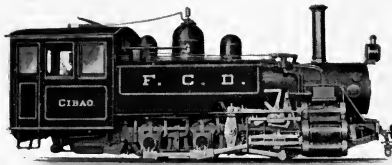
COMBINATION RACK AND ADHESION LOCOMOTIVE.
