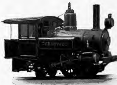
RACK LOCOMOTIVE, RIGGENBACH SYSTEM.
