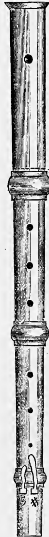
Fig. 31.—Flute of Quantz showing separate Keys for D♯ and E♭, enlarged from the Drawing in his Essay.
