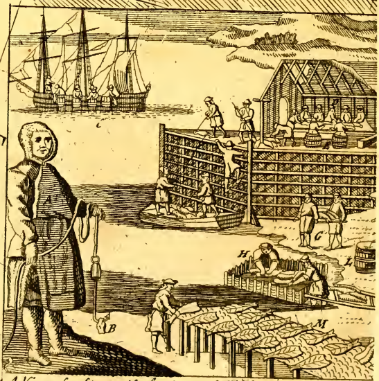
A View of a Stage, also of manner of Fishing for, Curing & Dressing of NEW FOUND LAND. A. The Habit of the Fishermen. B. The manner of Fishing. D. The Dressers of the Fish. E. The Trough they throw the Cod when dressed. F. Salt Boxes. G. The manner of cleansing the Cod. H. The Cleansing of the Cod. I. A Press to extract the Oil from the Cod's Liver. K. A Cask to receive the Water and Blood
