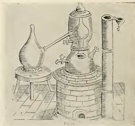
FIG. 58.—Furnace for Distillation.
