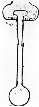
FIG. 51.—Apparatus for Distillation per Descensum . (Syriac MS.)
