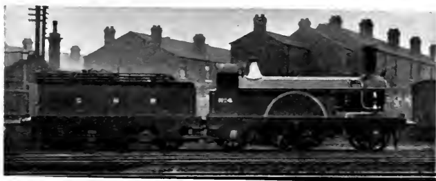
EXPRESS PASSENGER ENGINE "7' 0' SINGLE." BUILT FROM MR. STIRLING'S DESIGNS IN 1868.
