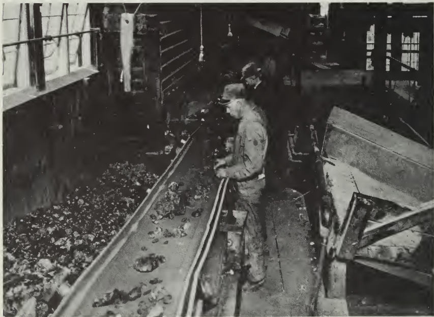
Removal of waste material from crude (fluorspar-zinc-lead) ore by hand-picking in the mill of Fairview Fluorspar & Lead Co., near Rosiclare, Illinois, 1919.
