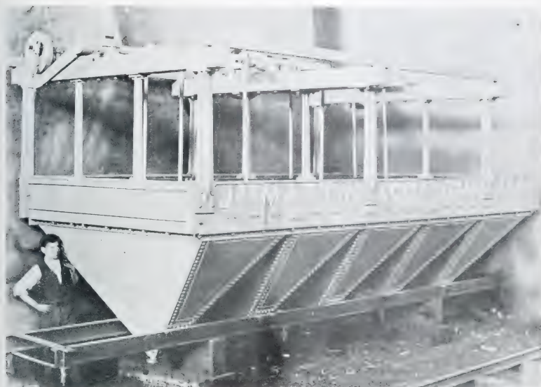
A Double Four-Hutch Plunger Jigger, manufactured by Jas. Martin & Co., Ltd.
