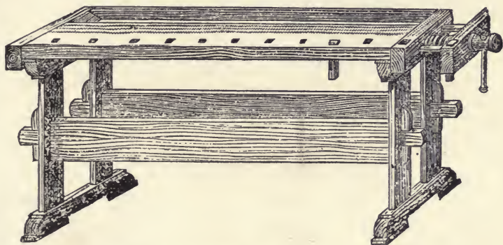
FIG. 24. SLOYD SCHOOL BENCH DESIGNED AT NÄÄS From Salomon: The Teacher's Handbook of Sloyd
