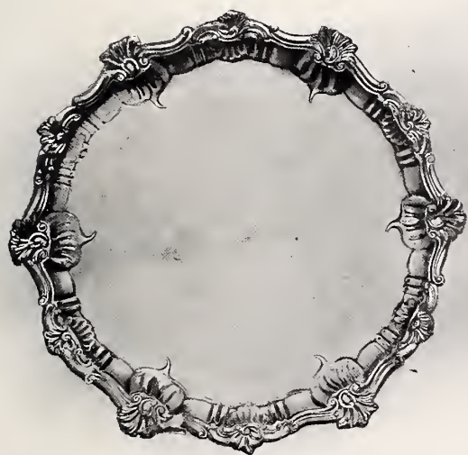
Front view of 8 in. Salver, made entirely by the aid of hand chasing. The general unevenness of the article will be noticed (see page 102). Date 1760.
