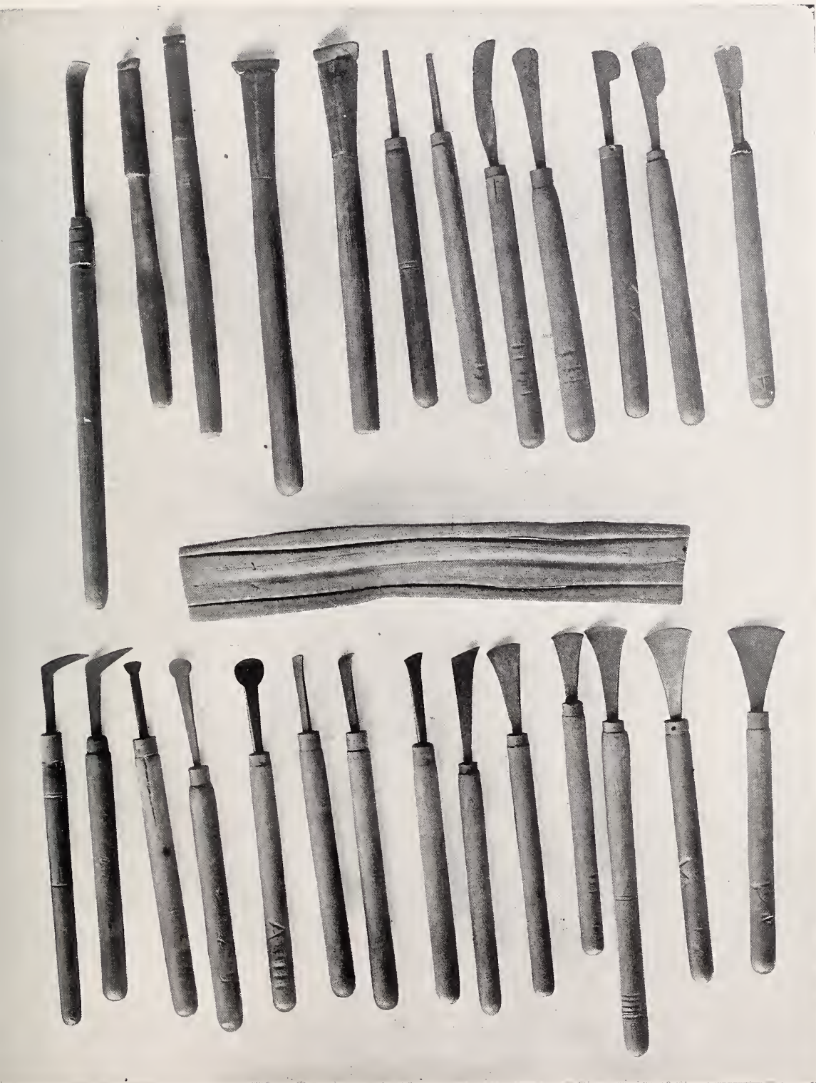
Illustrations of Burnishing Tools, showing the leather strop on which the burnish is constantly rubbed during the process. The marks on the handles are made by the various owners of the articles.
