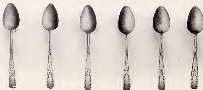
Tea Spoons, shanks made from plated drawn wire, and chased by hand, the bowls struck from a die and soldered on separately, by T. Law & Co.
