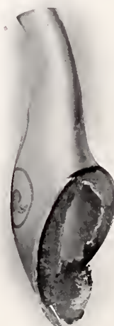
Teapot Spout, made of German silver, electro-plated. This has dropped off after 30 years' wear owing to decomposition referred to by Mr. A. S. Johnstone (see Page 139). The illustration is also instructive as showing how the tannin in the teapot spout will accumulate until finally it entirely chokes up the passage.
