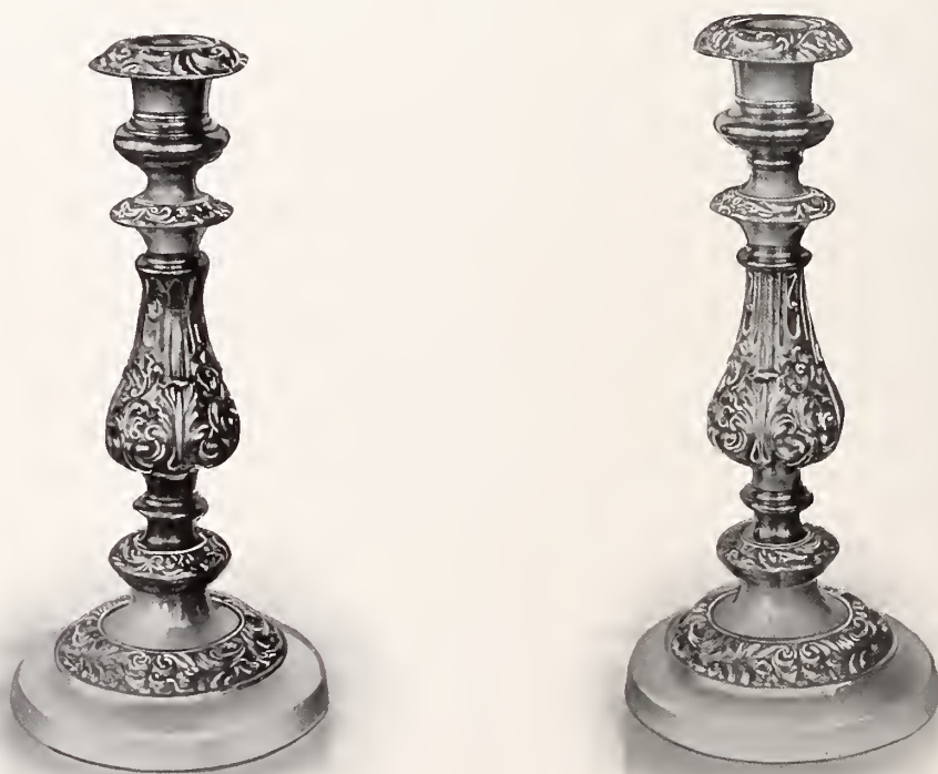
Specimen pair of the commonest quality 12 in. Candlesticks, showing that the silver has been worn completely away from every part of the sticks—the mounts show nothing but the mixture of lead and tin, other parts bright copper. Made in Birmingham, period
