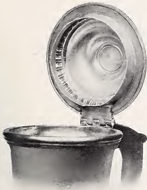
Early Coffee Pot, made before the invention of plating wire, showing the method of turning over the outer edge of lid to form a mount and secure the bizzle. The body is also turned over on the top to form a mount and to strengthen the article. Date 1758-1768. Author.
