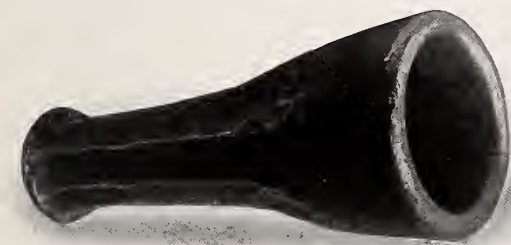
Drafting Punch, 8\frac{3}{4} in. long, 4 in. across mouth, being used by the stamper in forefront of illustration on next page.
