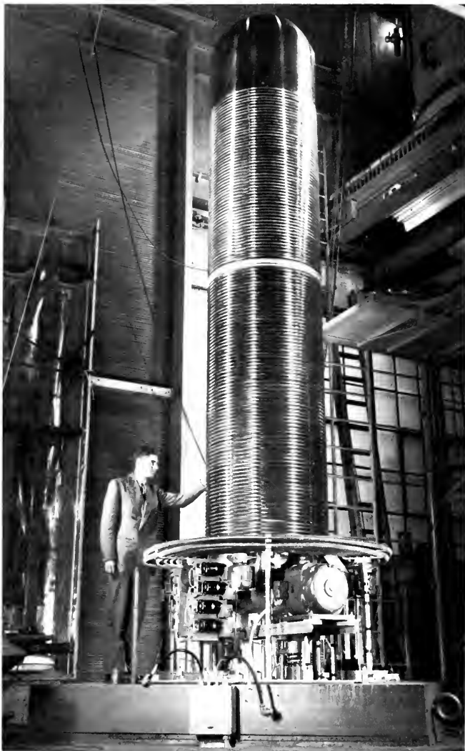
129. A view of Rice's Van de Graaff particle accelerator—the high voltage column, with the pressure tank removed.
