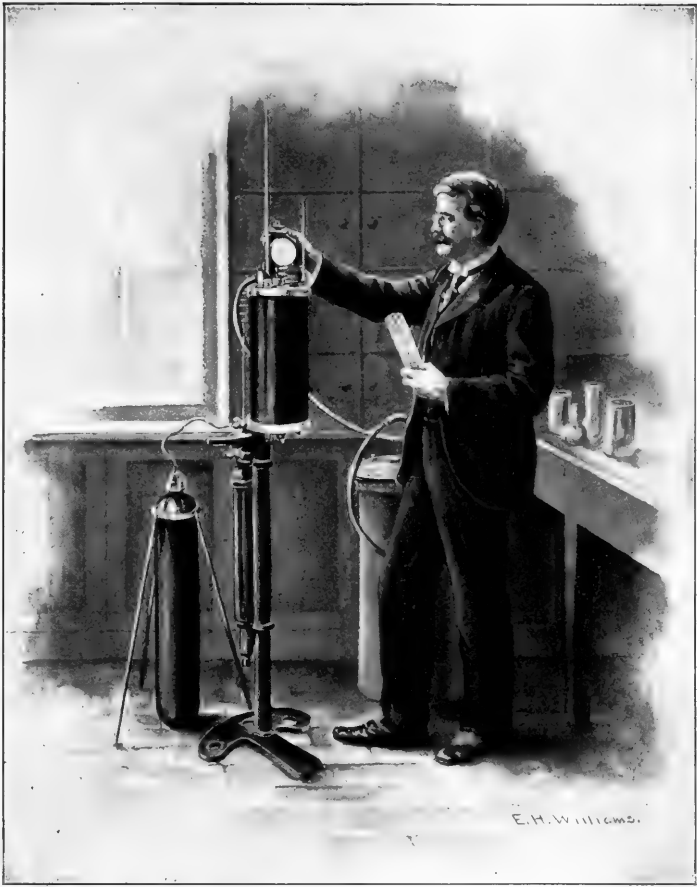
HAMPSON'S APPARATUS FOR LIQUEFYING AIR
