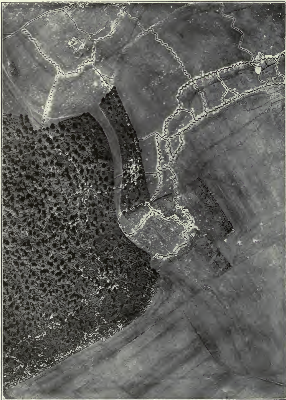
German--built trenches in the woods and in the open, part of Hindenburg Line N. W. of LIMEXY, France--note the numerous shell holes. Air photo, taken August 25, 1918, noon, at height of 3,000 meters
