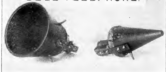
FIRST BELL TELEPHONES, PHOTOGRAPHED FROM THE ORIGINAL INSTRUMENTS IN THE PATENT OFFICE AT WASHINGTON
