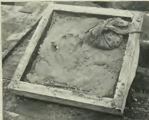
FIG. 9. TAMPING THE SAND INTO PLACE IN THE PLASTER MATRIX.
