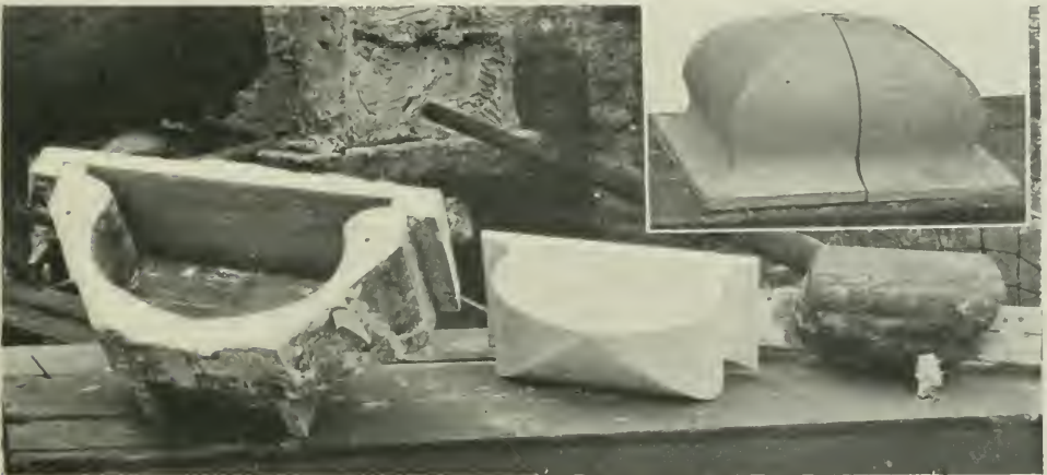
FIG. 28. CASTING THE HOLLOW PLASTER BLOCK IN HALVES.
