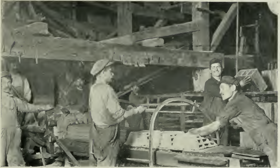
FIG. 2. WHERE THE CLAY STREAM IS CUT INTO BLOCKS.
