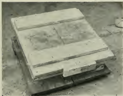
FIG. 12. THE WOODEN MATRIX, WITH THE PALETTE COVERING IT.
