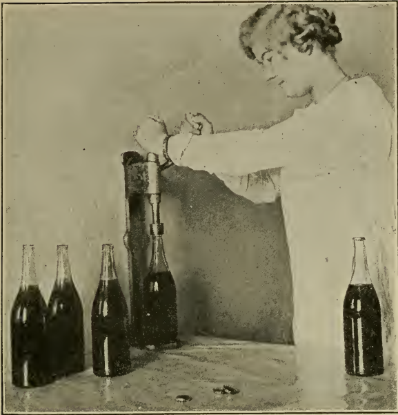
FIG. 24. Capping Bottles with Small Hand Power Crown Capper. Note that bottles are not completely full.
