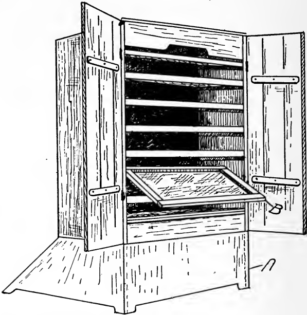
FIG. 45. Small Home Made Cabinet Dryer. Can be used on kitchen stove.
