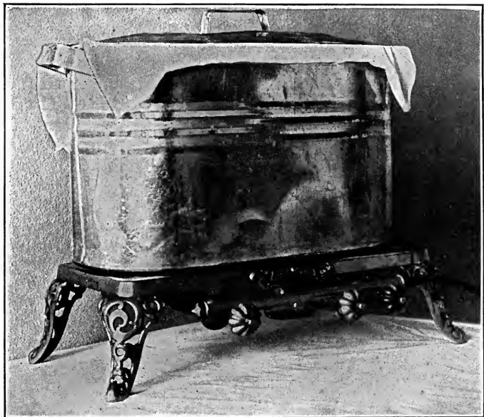
FIG. 15. Washboiler Sterilizer with Cover Made Tight by Use of a Cloth. This is a very effective method of covering boilers that have poorly fitting covers.
