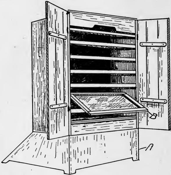
FIG. 45. Small Home Made Cabinet Dryer. Can be used on kitchen stove.
