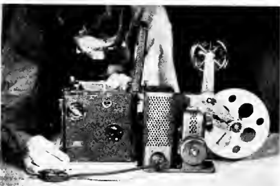
Fig. 1. The owner of a reflex camera can use it for vertical projection.
