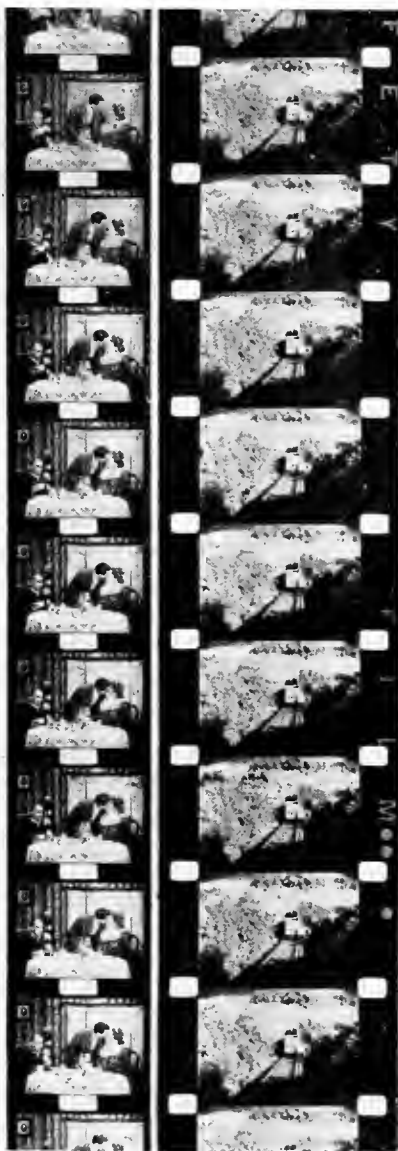
An interesting comparison. Enlarged pictures of strips of 9½ and 16-mm. films to same scale. Notice that, contrary to common opinion, for the same number of pictures or time on the screen, the 9½-mm. film is just as long as the 16-mm. (See article on page 12.)
