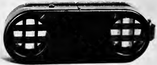
Above.—A rear view of the meter, showing the two photoelectric cells and the angle-correcting shades
