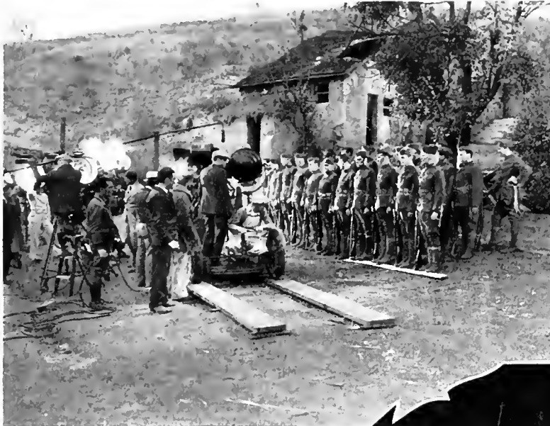
From "Private Jones," showing camera "dolly" and use of artificial light to aid daylight (Universal)
