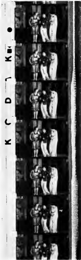
A strip of R.C.A. 16 mm. talkie film Note the sound track on the right
