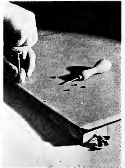
Above, Fig. 3. Screw one edge of the screen to a length of wood batten. In the ends of the batten fix the two long screws
