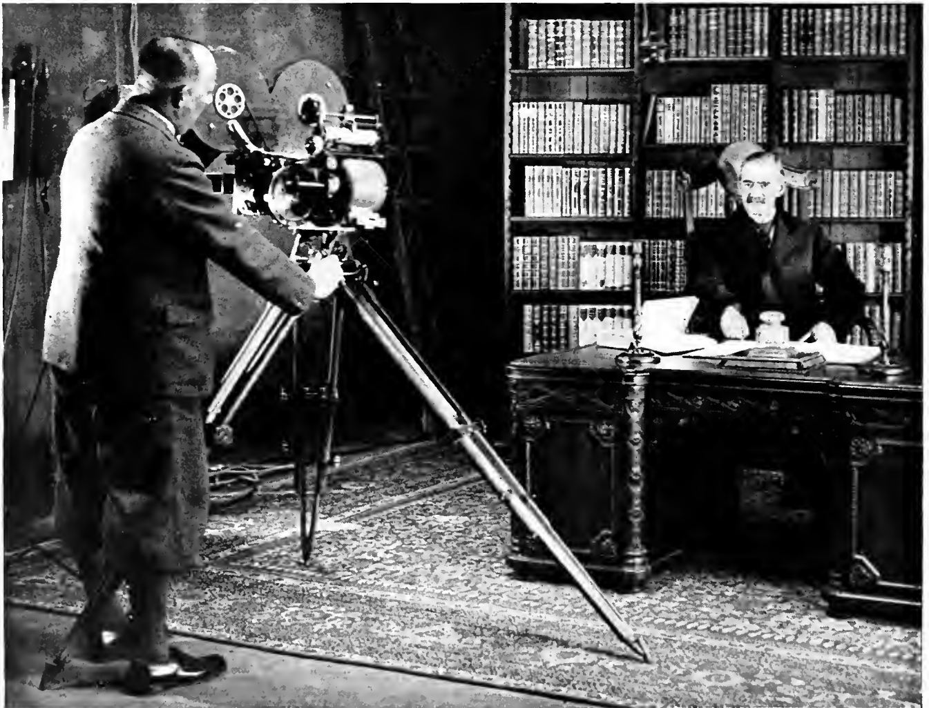
Making a talkie film of Mr. Neville Chamberlain. The camera is motor driven by current from the nearest light socket, while the microphone can just be seen suspended above the table in front of the top row of books. Large portable lights are used to give additional illumination
