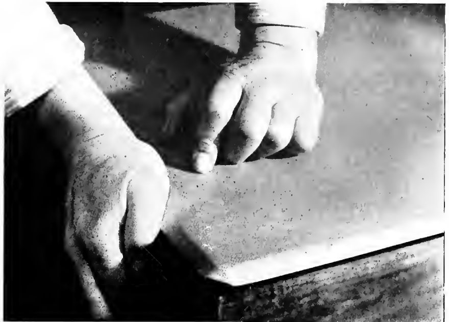
Fig. 4. Bending the edges of the aluminium sheet over the edge of a table like this will make it much stiffer
