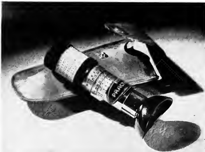
★ The Practos exposure meter is marked for use with either still or cine cameras
