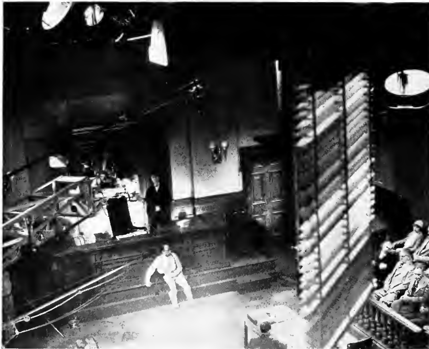
An example of how the Cameraman has to watch the microphone boom. The two microphones shown must be placed as near the artists as possible, but must be kept clear of the camera's line of vision. (From the Paramount film, "The Night of June 13.")
