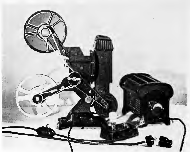
Here is the complete outfit with pilot light and resistance for 200-250 volts
