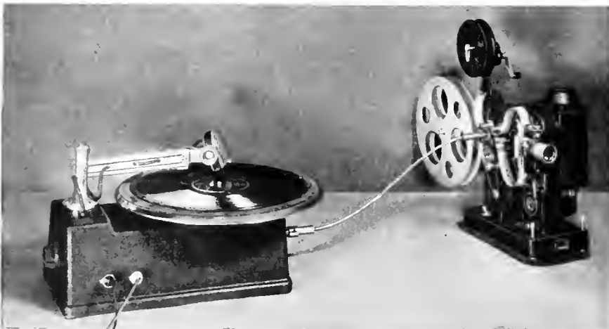
Fig. 2. A simple home talkie outfit using a synchronised turntable driven from a 16-mm. projector (Courtesy A. W. Green)
