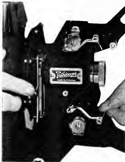
The gate is opened by a touch of the finger (on the left). On the right the take-up sprocket guard is being lifted
