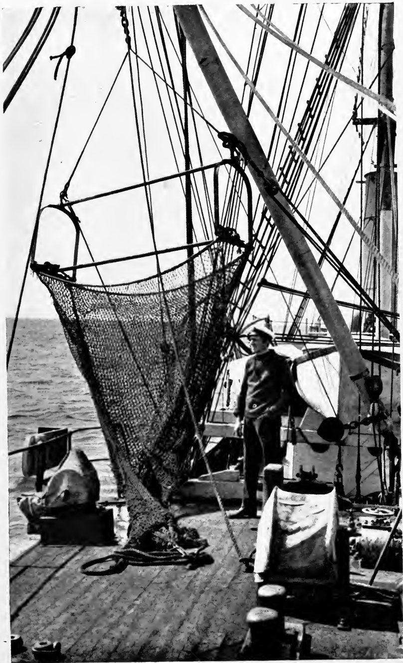
THE MONAGASQUE TRAWL HOISTED ON THE DERRICK : GRAY STANDING BY
